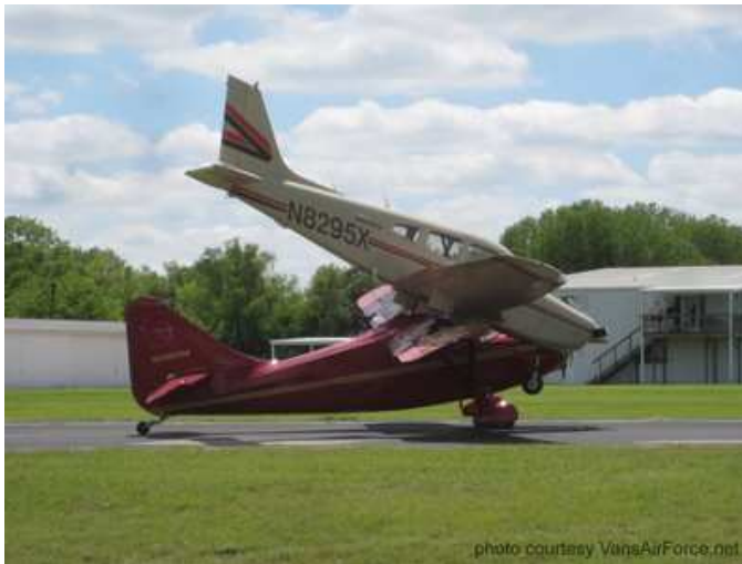
Figure 1.2: Example: An accident happened where a low-wing aircraft landed on top of a high-wing aircraft, because the wings prevented visual separation. Luckily there were no injuries in this case.
