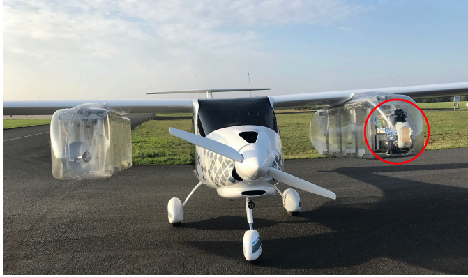
Figure 5.11: The test aircraft, with the radar in the port freight container
