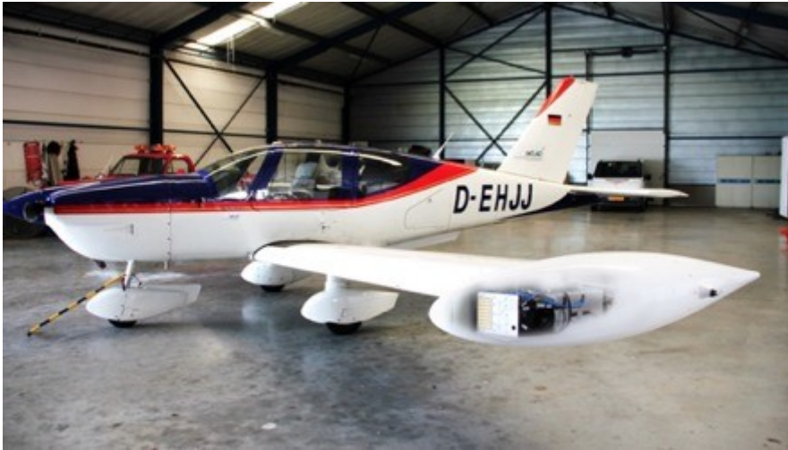
Figure 6.1: The test aircraft with the radar in the wingtip
