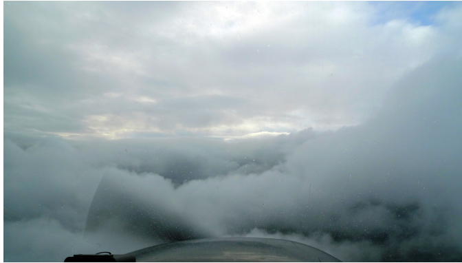
Figure 1.1: Instrument Meteorological Conditions in which eyesight is hindered and VFR cannot be applied safely
