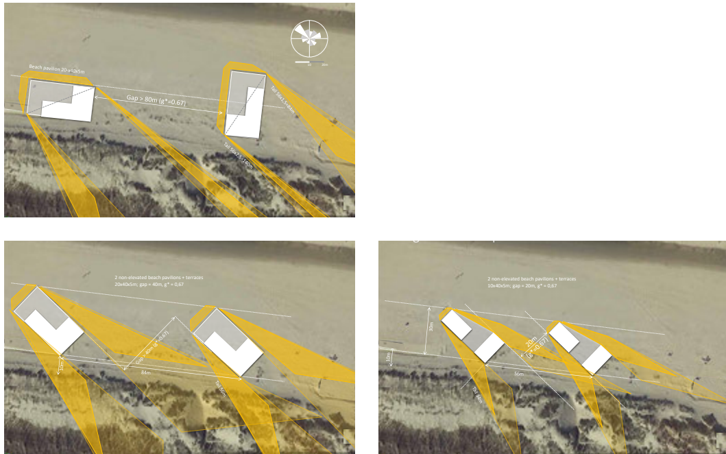
FIG. APP.A.16 Overview (PO (top), P1 and P2 (right)) of the principal sand-tail development of beach pavilion configurations in the dominant wind direction promoting dun- widening. Images by the author. Aerial photograph: Google Earth.
