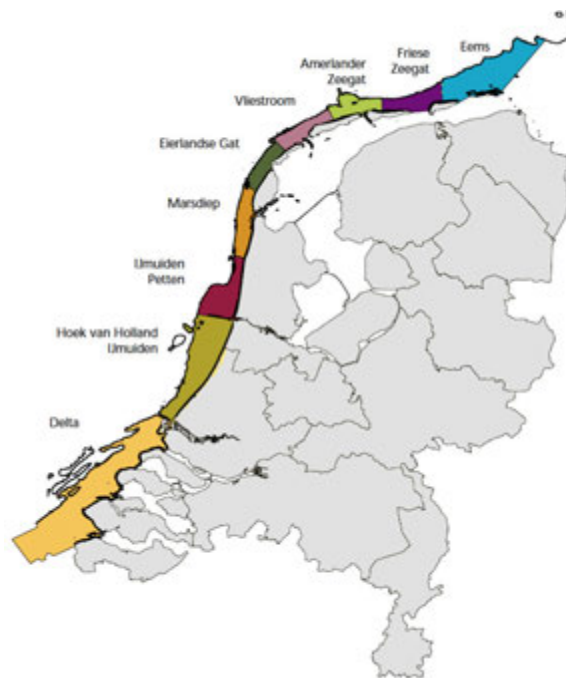
FIG. 3.2 Map of the Dutch coast divided into coastal cells, each with specific dynamics and sediment needs. Source: Mulder, 2000.
