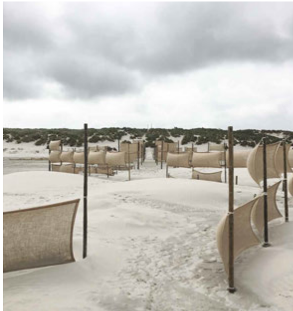
FIG. 3.54 Sand tail deposition by blowouts in the fences. Source: LA students TU Delft, 2018.
