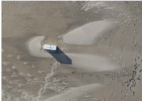
FIG. 3.22 Day accretionary pattern around a scale model during fieldwork. Source: Poppema et al., 2019.
