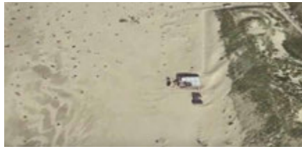
Downwind sand tail development behind beach buildings in Hargen, North-Holland.
