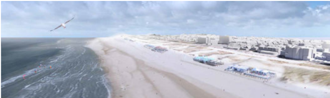
b) Noordwijk as a Dike in dune plus-, or Sand buffer phase 1 reinforcement, promoting BwN-based dune heightening
