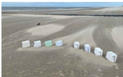
FIG. 3.71 (right) Field test of a V-shaped scaled row house configuration on an open beach plain in Vlieland (2020), combining wind convergence and oblique placement to lengthen tails and guide sediment to the back as an artificial blowout. Image by the author.
