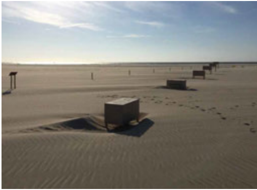
FIG. APP.A.4 Photograph of the sand-tail patterns behind scale models B1, B2 and B3 after 6 weeks, with the downwind deposition tails clearly visible (left). Source: J. van Bergen.
