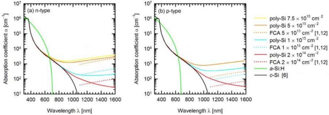
Figure 3.4 The absorption coefficient as a function of the Wavelengths. (a) For n+ poly-Si layer (b) for p+ poly-Si layer [47].
