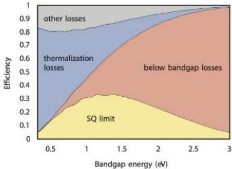
Figure 1.5 SQ limit along with the major losses for AM1.5 spectrum [5].
