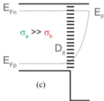
A heterojunction is formed between c-Si and a wider bandgap material. Here there is a proper alignment of the conduction bands to facilitate electron selectivity. In reality, this is not the case and we have to try keeping the off-set between the conduction band (in case of electron selectivity) sufficiently small, with fermi level alignment.
