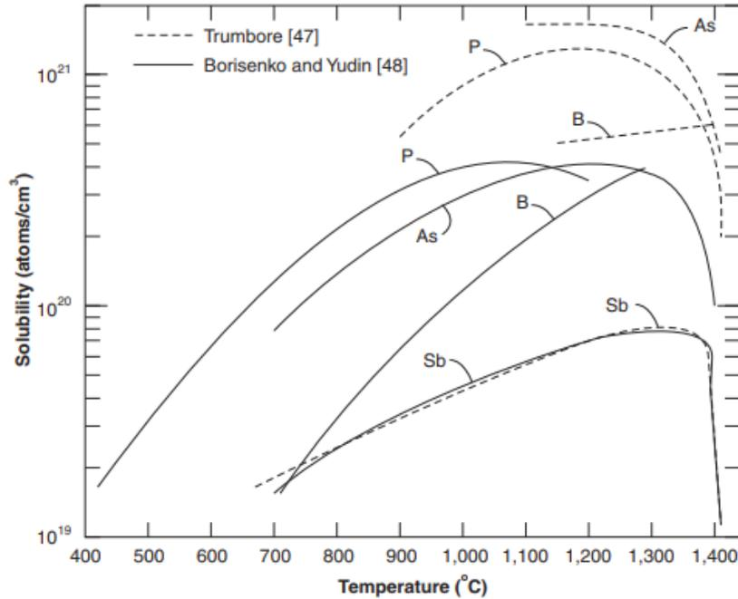
Figure 3.5 Solubility of dopants in silicon as a function of temperature [49].
