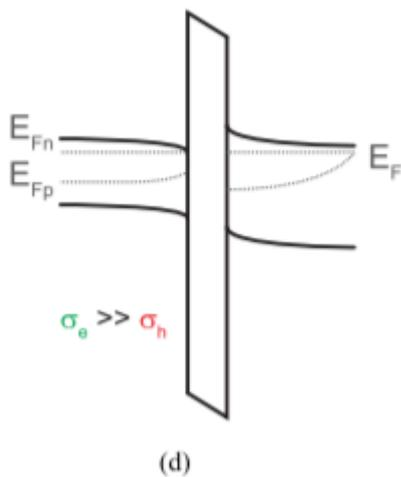
A tunnel layer, ultra-thin SiO<sub>x</sub> layer is introduced between the n and a heavily doped n<sup>+</sup> layer, which has an asymmetric probability of the electrons and holes to tunnel through. The SiO<sub>x</sub> layer provides better tunnelling for electrons compared to that of holes. This type of CSCs are used in this thesis work with thermal SiO<sub>x</sub> enabled by poly-Si.
