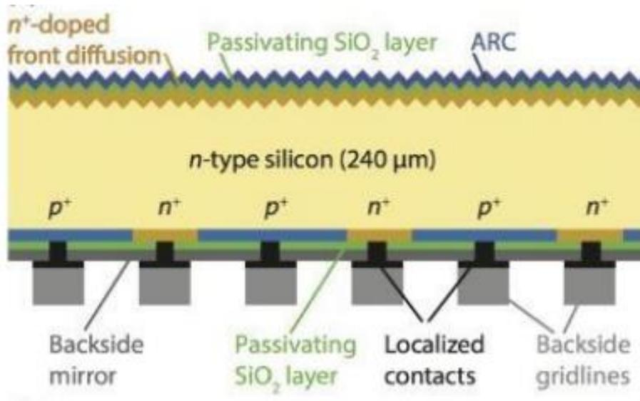
Figure 1.8 IBC solar cell architecture [5].
