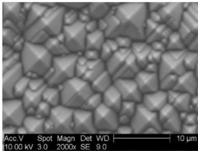
Figure 2.1 Textured c-Si surface under SEM [13].
