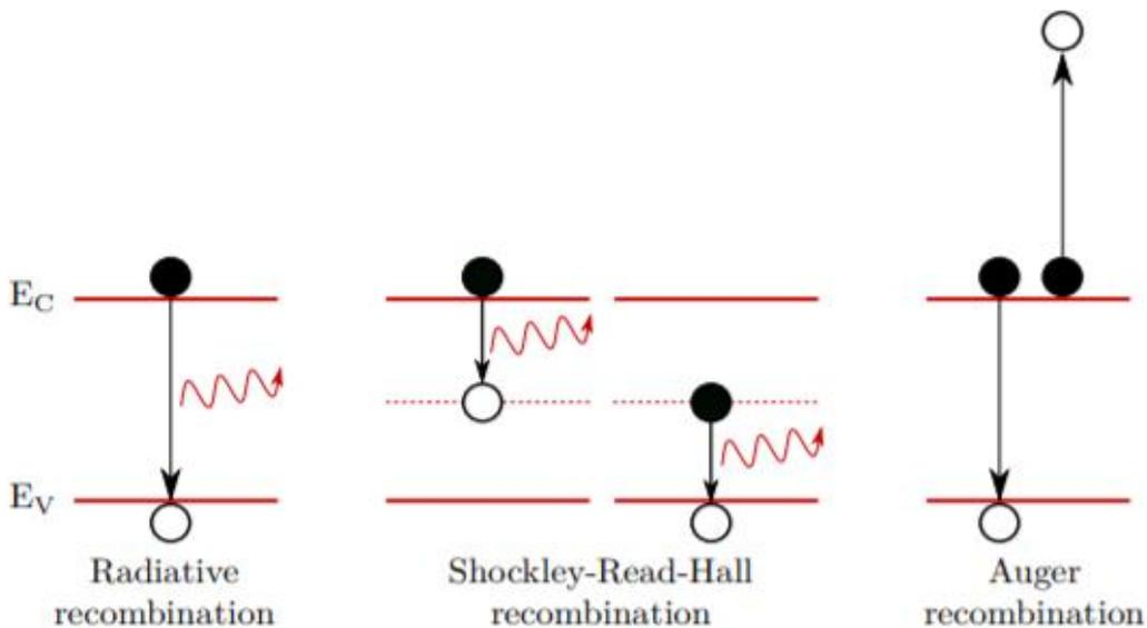
Figure 1.4 Schematic of recombination mechanism [6].
