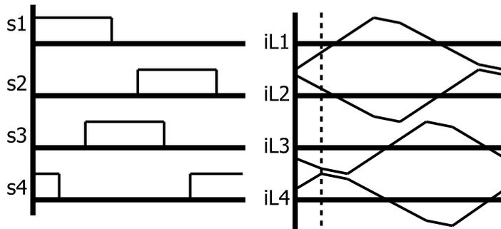
Figure D.3: Switching patterns and inductor current ripple in the CIIBC.
