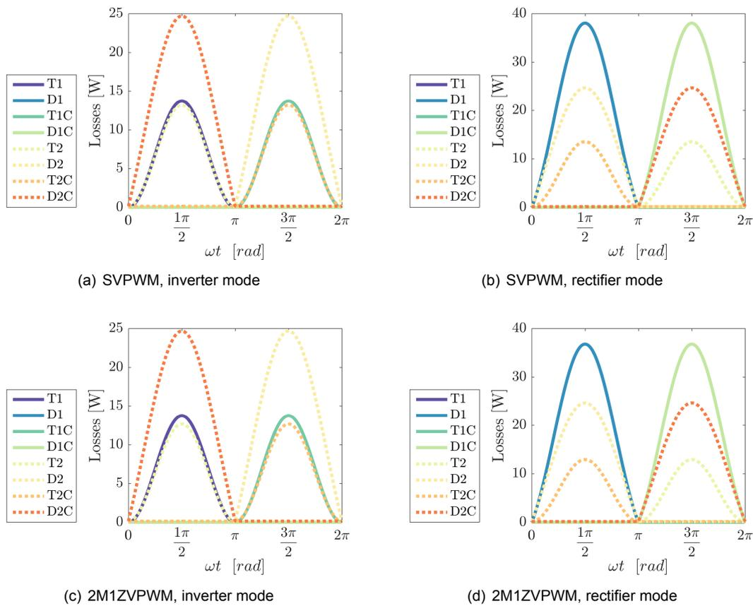
Figure 7.32: Conduction losses of the 3LT<sup>2</sup>C,  $F_{sw} = 50$  kHz
