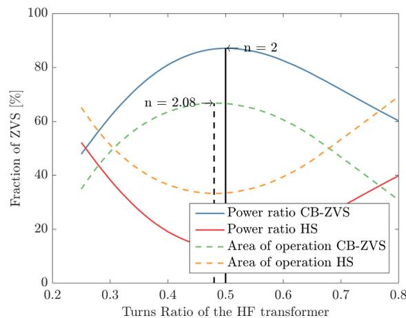
Figure 6.6: Optimum turn ratio for the two optimization approaches for the DAB,  $L = L_{Leak}^{opt}$
