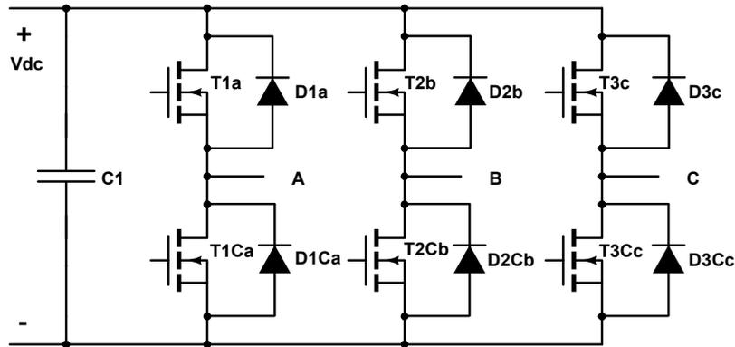
Figure 2.12: Structure of the 2LC
