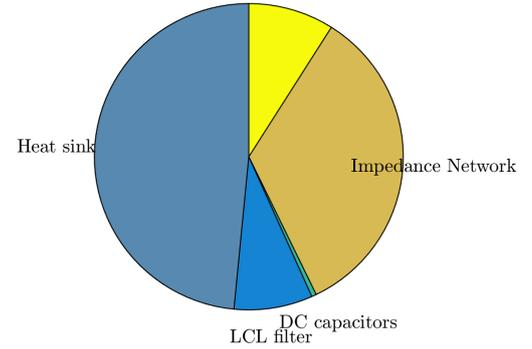
Fig. 22: Size distribution of the quasi Z-Source Inverter (qZSI).
