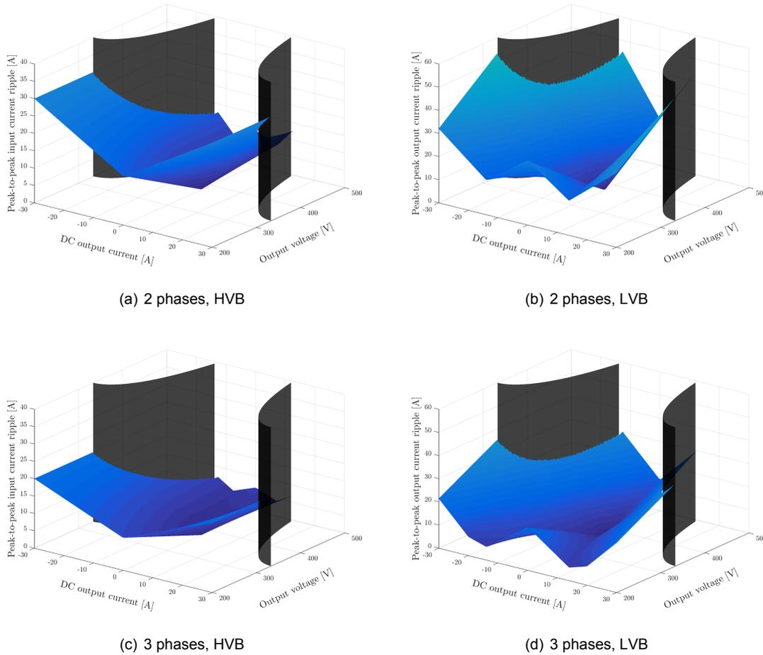
Figure 6.7: Current ripple at both bridges of the DAB
