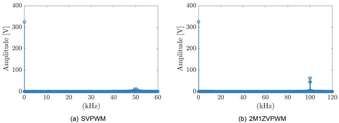
Figure 7.23: FFT of the 3LNPC<sup>2</sup> for both modulation techniques.  $F_{sw} = 50$  kHz
