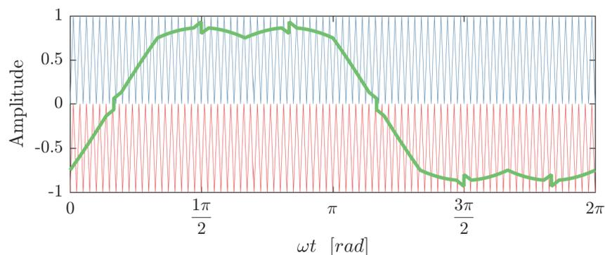
Figure 7.21: Reference waveforms and carrier signal of the 2M1ZVPWM
