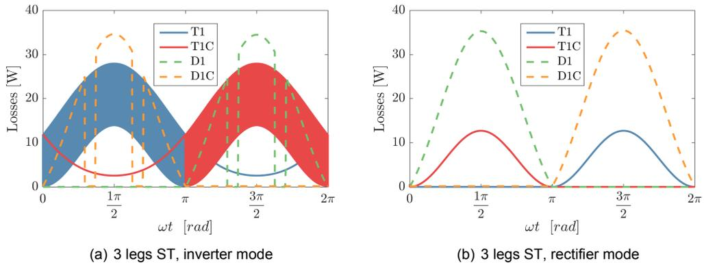
Figure 8.5: Conduction losses of the qZSI,  $F_{sw} = 50$  kHz
