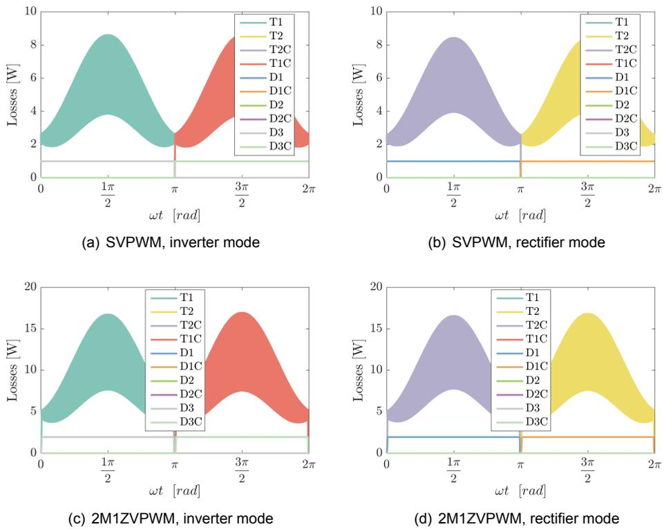
Figure 7.26: Switching losses of the 3LNPC<sup>2</sup>,  $F_{sw} = 50$  kHz
