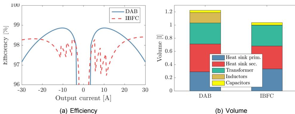
Figure 6.22: Results of the optimal topologies configurations of the PV port.
