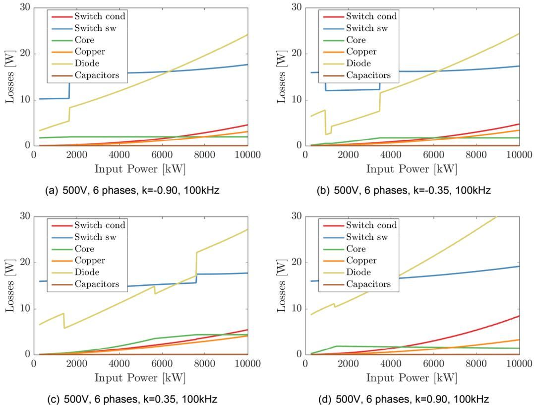
Figure 5.15: Losses versus input power on the different elements at 500 V
