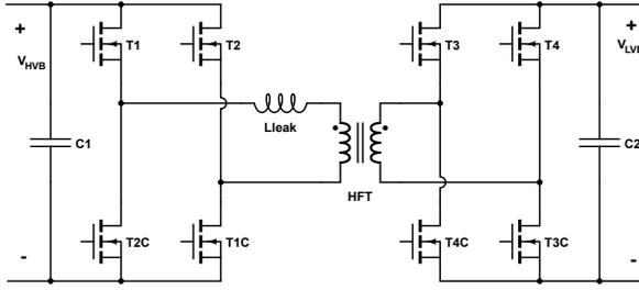
Fig. 11: Structure of the DAB
