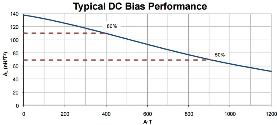
Figure 4.3: DC Bias performance example of Kool Mu 0077192A7 toroid. Source: Datasheet
