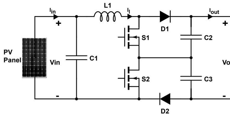
Figure 2.8: Structure of a one phase TLBC
