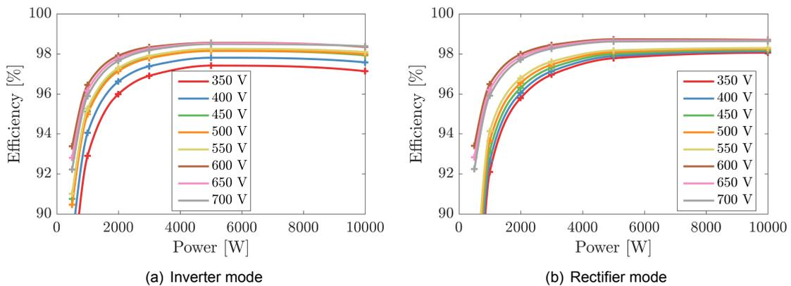
Figure 8.8: Efficiency of the qZSI at different operating points.
