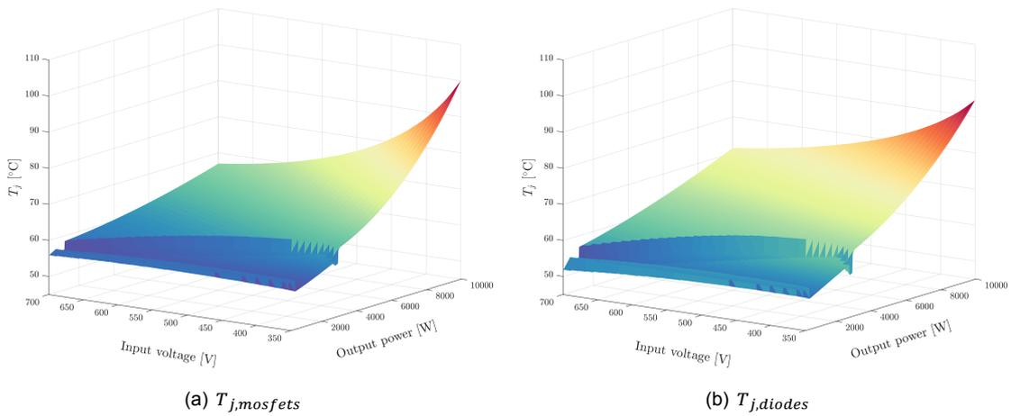
Figure 5.17: Junction temperatures of CIIBC (4 phases 50 kHz example)
