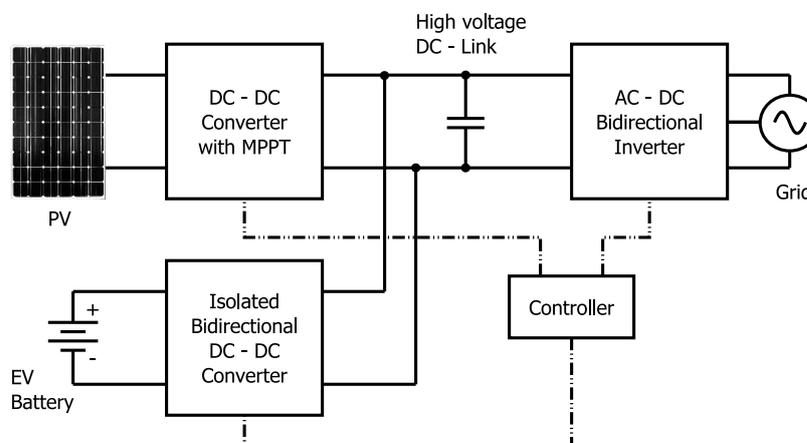
Figure 2.2: Block diagram of a three-port converter with a DC link
