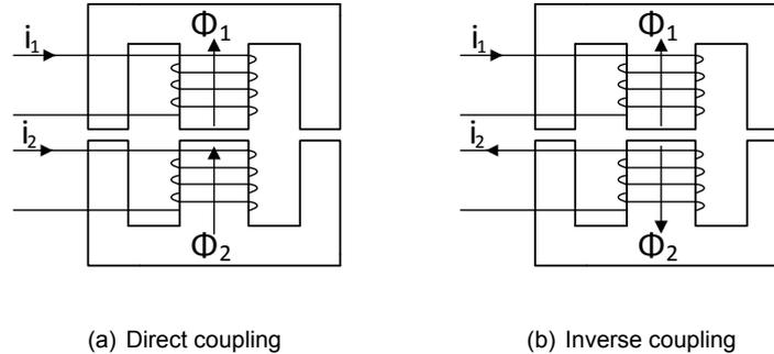
Figure 5.11: Coupling configurations in an E core
