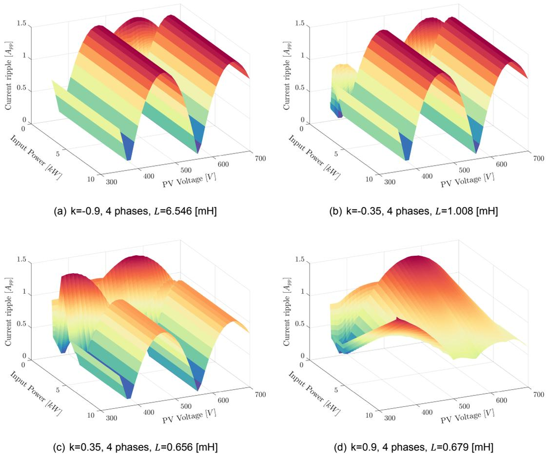
Figure 5.13: Input ripple in the CIIBC for 4 phases and different coupling factors
