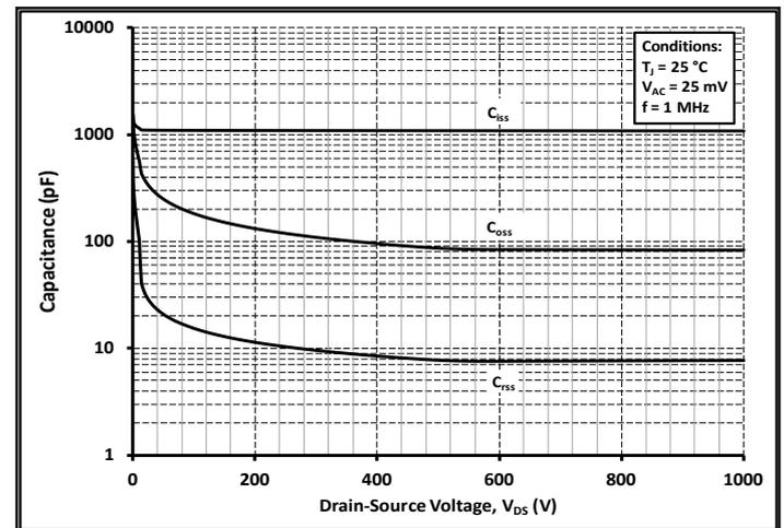
Figure 18. Capacitances vs. Drain-Source Voltage (0 - 1000V)
