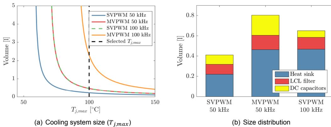
Figure 7.36: 3LT<sup>2</sup>C system size
