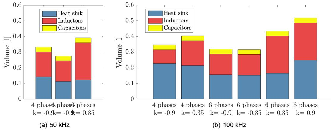
Figure 5.18: Volume of the different possible configurations of the CIIBC
