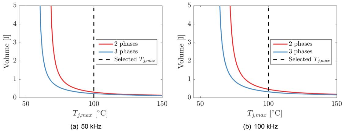
Figure 5.26: TLBC cooling system size for different values of  $T_{j,max}$
