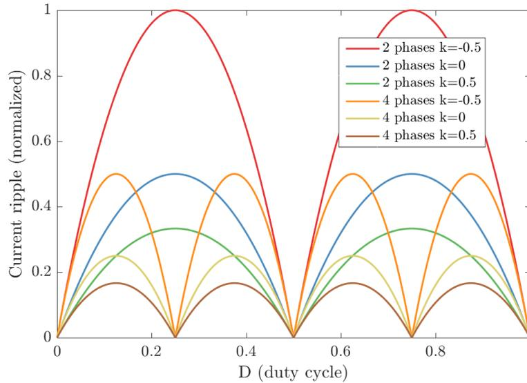
Figure 5.12: Input current ripple versus duty cycle for different levels of interleaving
