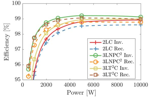
Fig. 18: Efficiency of the Grid port candidates ( $V_p = 230V$ )
