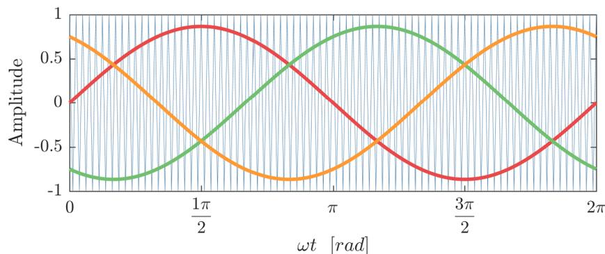
Figure 7.2: Sinusoidal carrier versus triangular wave in SPWM
