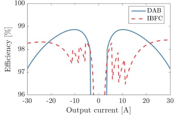
Fig. 13: Efficiency of the EV port candidates ( $V_o = 332V$ )
