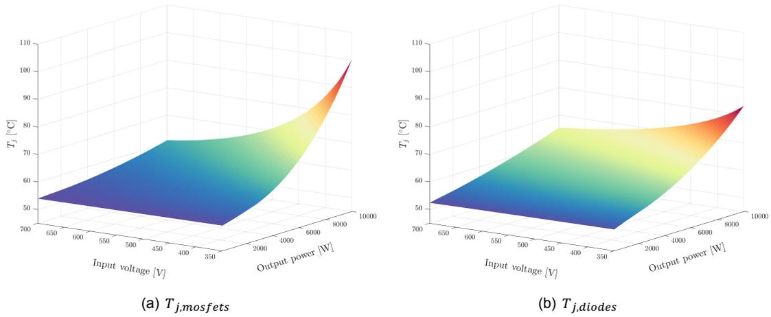
Figure 5.8: Junction temperatures of IBC (3 phases 100 kHz example)
