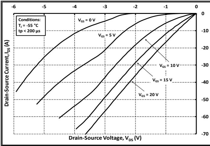
Figure 13. 3rd Quadrant Characteristic at  $-55\text{ }^\circ\text{C}$
