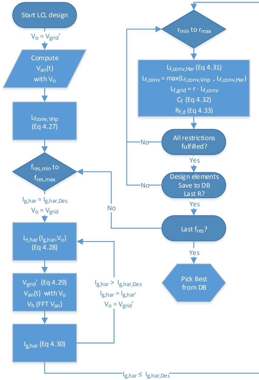
Figure 4.5: LCL filter design procedure
