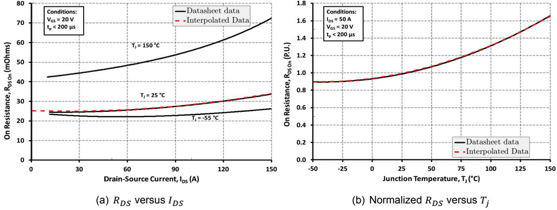
Figure 3.1: Example of an interpolation, superimposed to the datasheet (CREE C2M0025120D).
