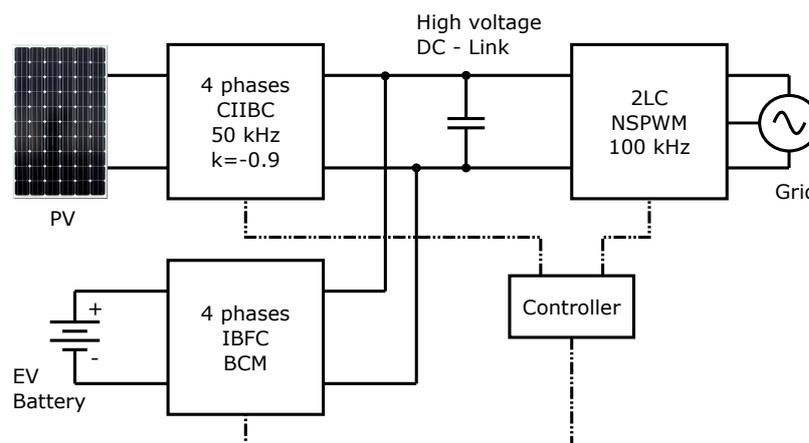
Figure 9.1: Block diagram of the final multiport converter
