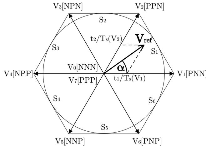
Figure 7.3: Working principle of the Space Vector Modulation (SVM)
