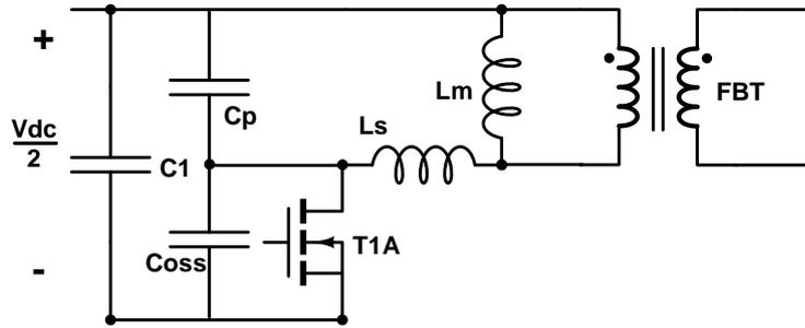
Figure 6.15: Parasitic elements present on the IBFC
