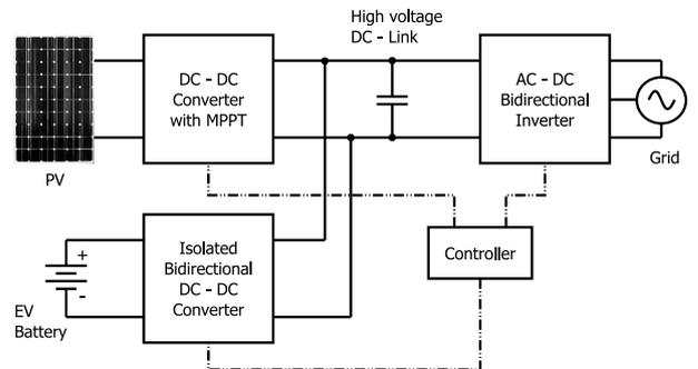
Fig. 2: Block diagram of a three-port converter with a DC Link.
