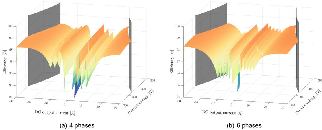
Figure 6.21: Efficiency of the four and six phases IBFC
