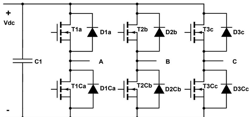
Figure 7.1: Structure of the 2LC
