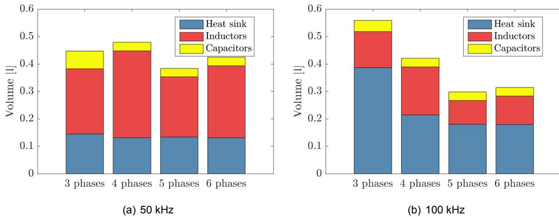
Figure 5.9: Volume of the different possible configurations of the IBC
