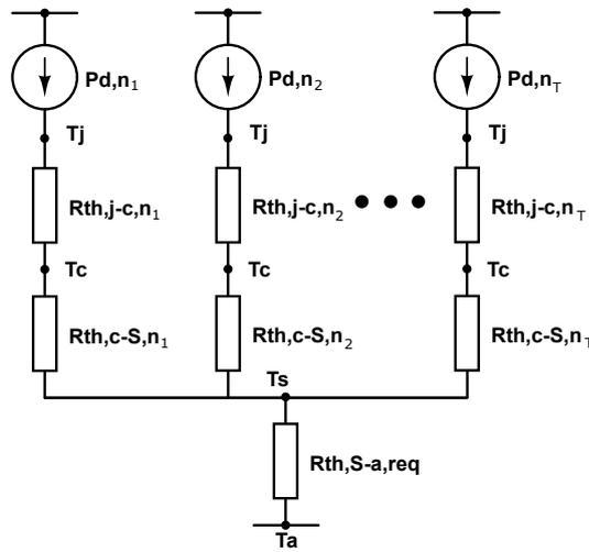
Figure 4.6: Equivalent thermal circuit model of the cooling system
