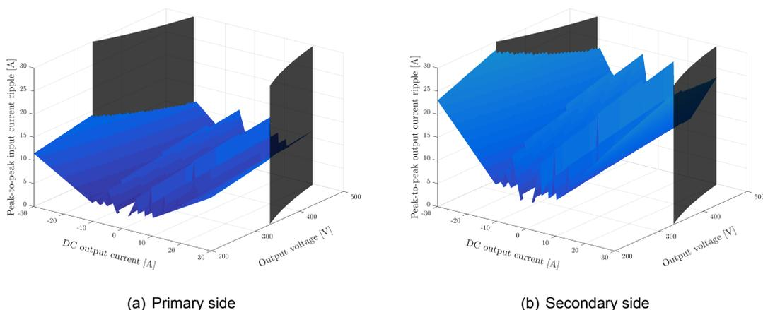
Figure 6.17: Current ripple at both sides of the 4 phases IBFC
