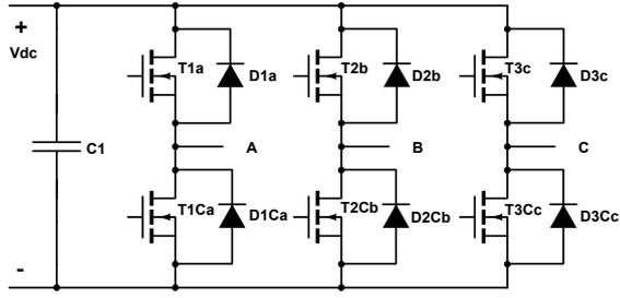
Fig. 15: Structure of the 2LC
