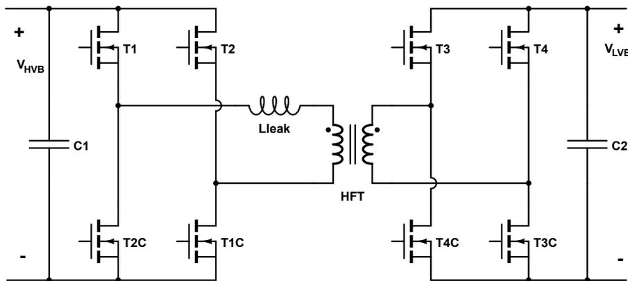
Figure 6.2: Structure of the of the DAB
