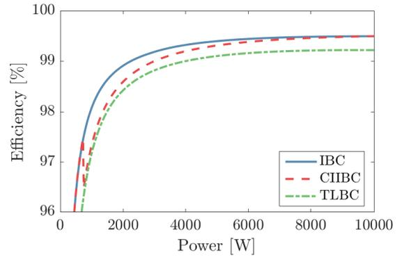
Fig. 9: Efficiency of the PV port candidates ( $V_i = 500V$ )
