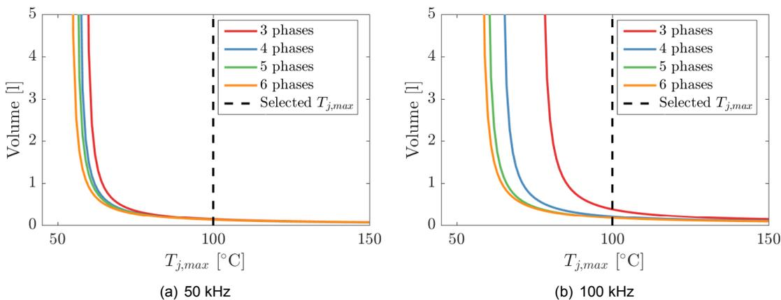
Figure 5.7: IBC cooling system size for different values of  $T_{j,max}$
