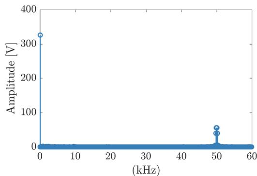
Figure 8.4: FFT of the qZSI at 50 kHz.
