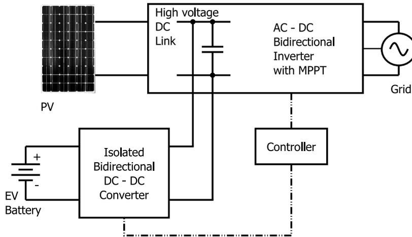
Figure 2.3: Block diagram of a three-port converter with an impedance network
