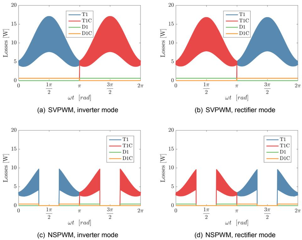
Figure 7.13: Switching losses of the 2LC,  $F_{sw} = 50$  kHz
