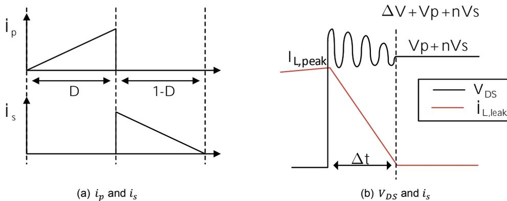
Figure 6.16: Voltage and current waveforms of the IBFC (charging mode)
