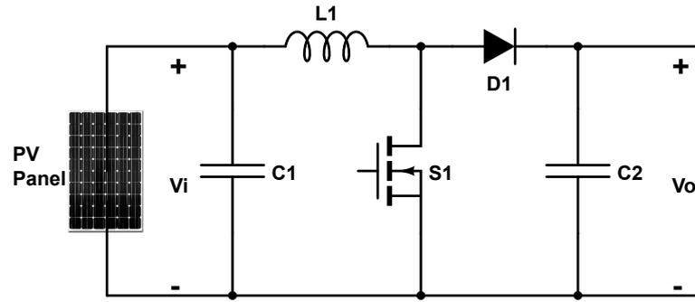
Figure 2.5: Structure of a boost converter
