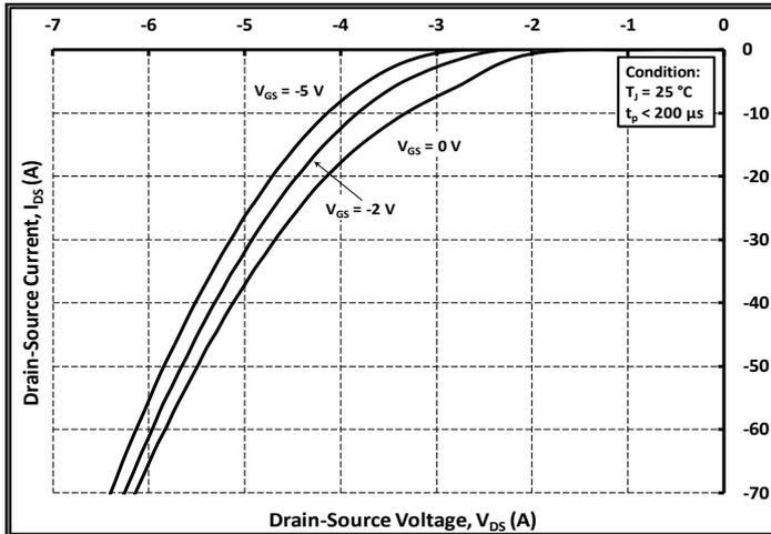
Figure 9. Body Diode Characteristic at  $25\text{ }^\circ\text{C}$
