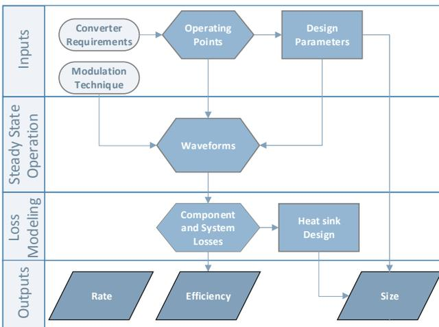
Fig. 1: Overview of the methodology used to rate every topology.
