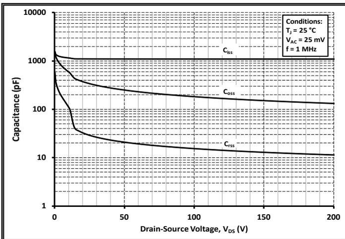
Figure 17. Capacitances vs. Drain-Source Voltage (0 - 200V)
