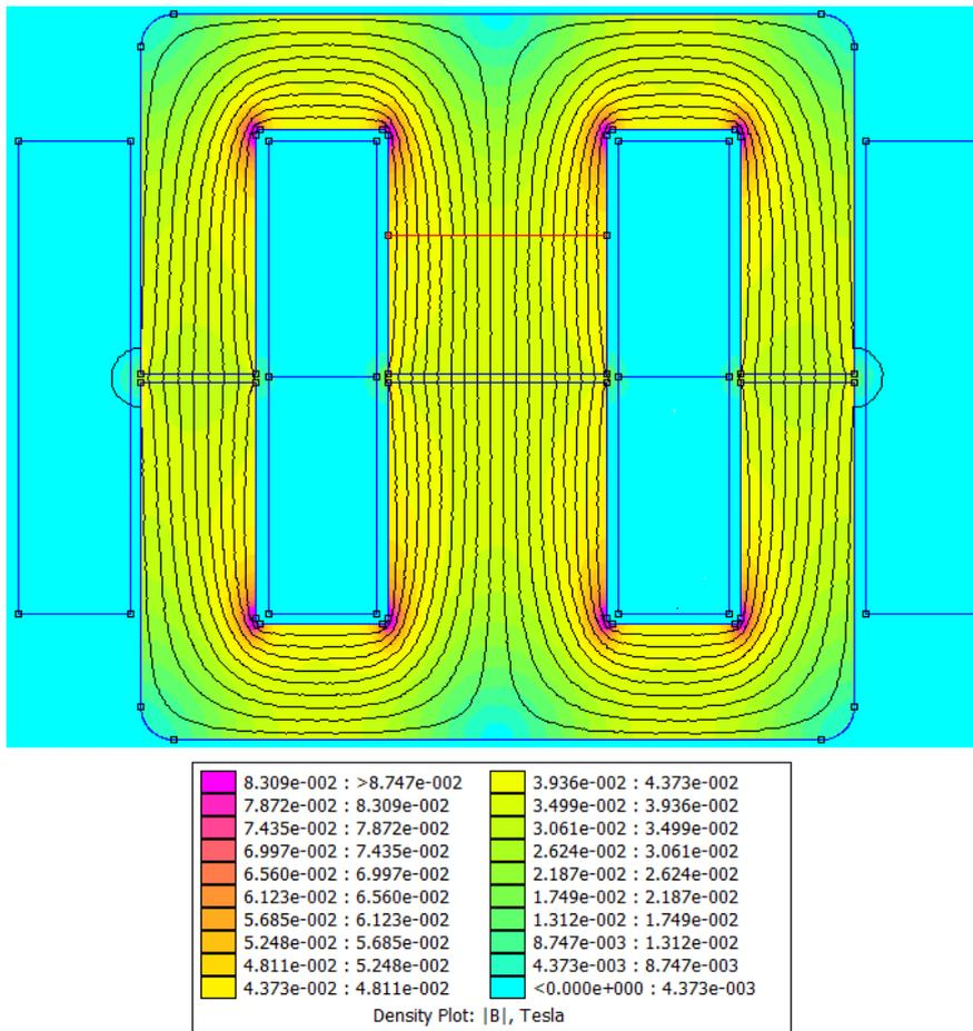
Figure B.3: FEM results of the 4 phases CIIBC inductor
