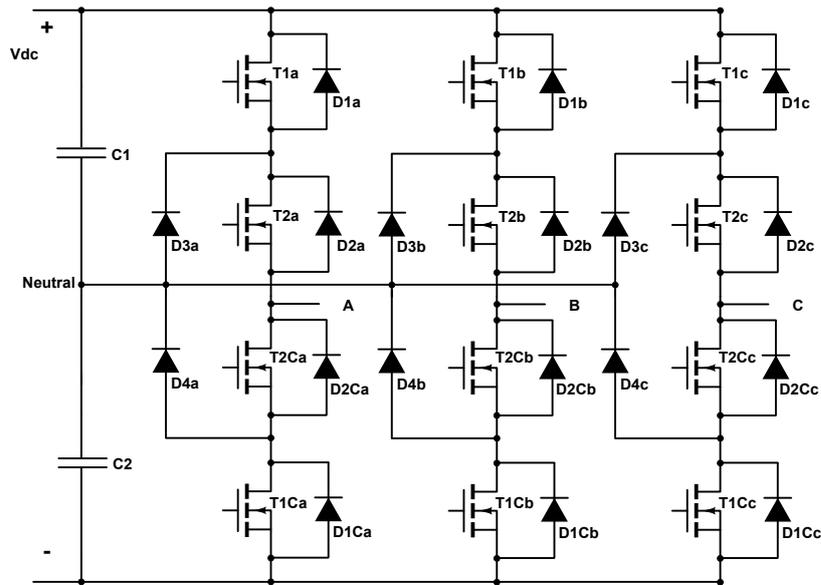
Figure 2.13: Structure of the 3LNPC<sup>2</sup>
