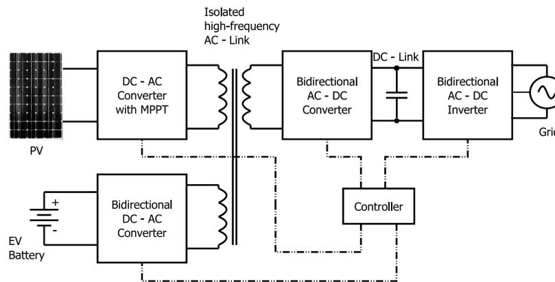
Figure 2.4: Block diagram of a three-port converter with an inner AC link.
