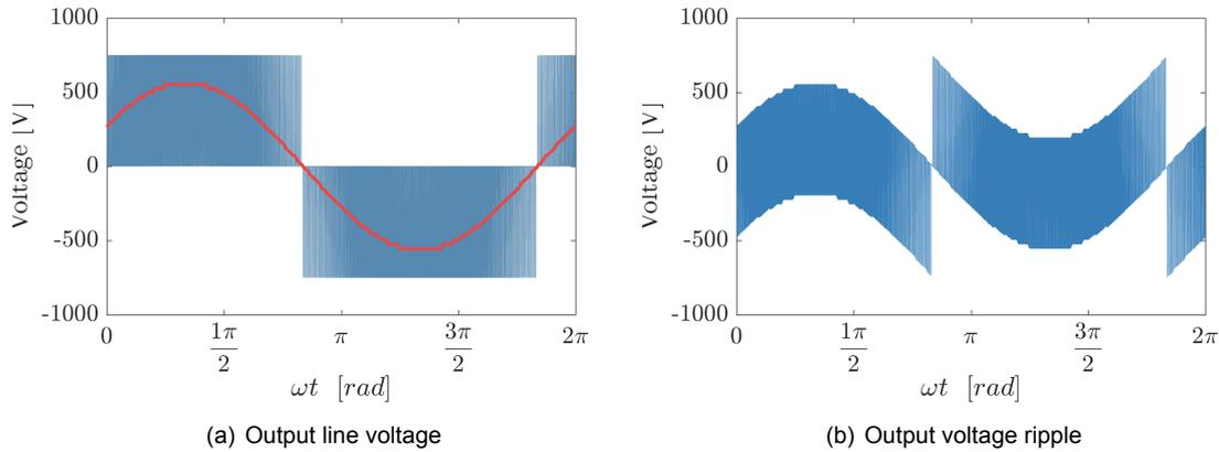
Figure E.4: Voltage waveforms of the 2LC using SVPWM.  $F_{sw} = 4kHz$
