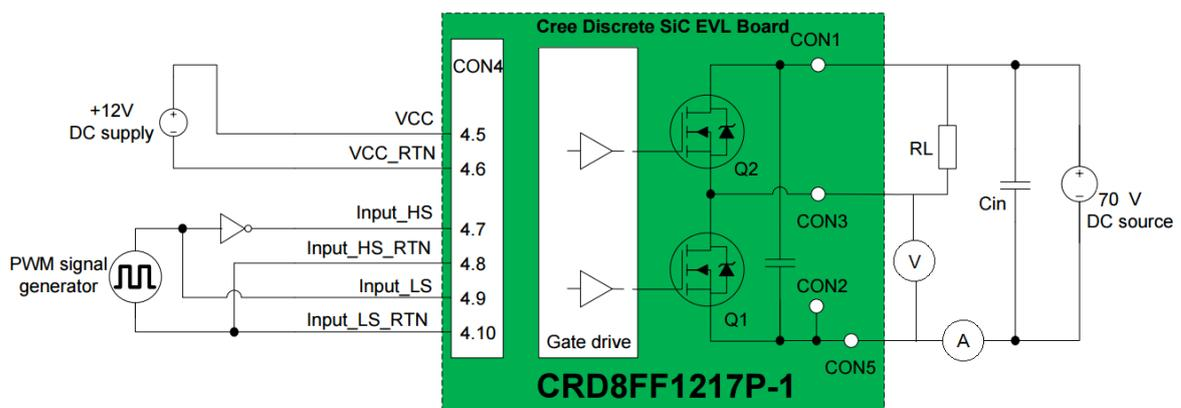
Figure C.1: Test setup of the evaluation board.
