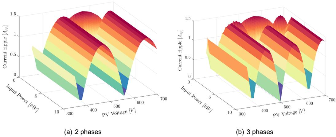
Figure 5.23: Input current ripple versus input voltage and power for different levels of interleaving
