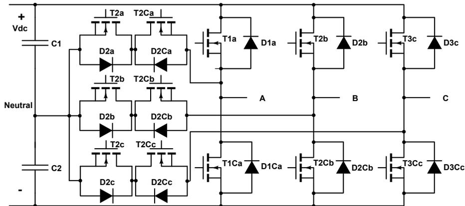
Figure 7.30: Structure of the 3LT<sup>2</sup>C
