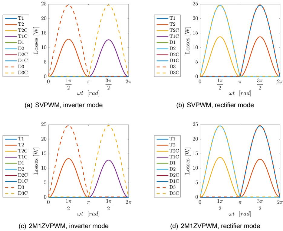
Figure 7.25: Conduction losses of the 3LNPC<sup>2</sup>,  $F_{sw} = 50$  kHz
