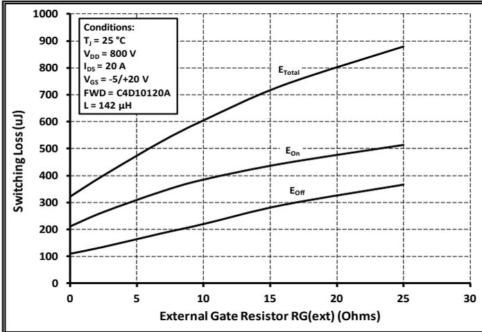
Figure 25. Clamped Inductive Switching Energy vs.  $R_{G(\text{ext})}$
