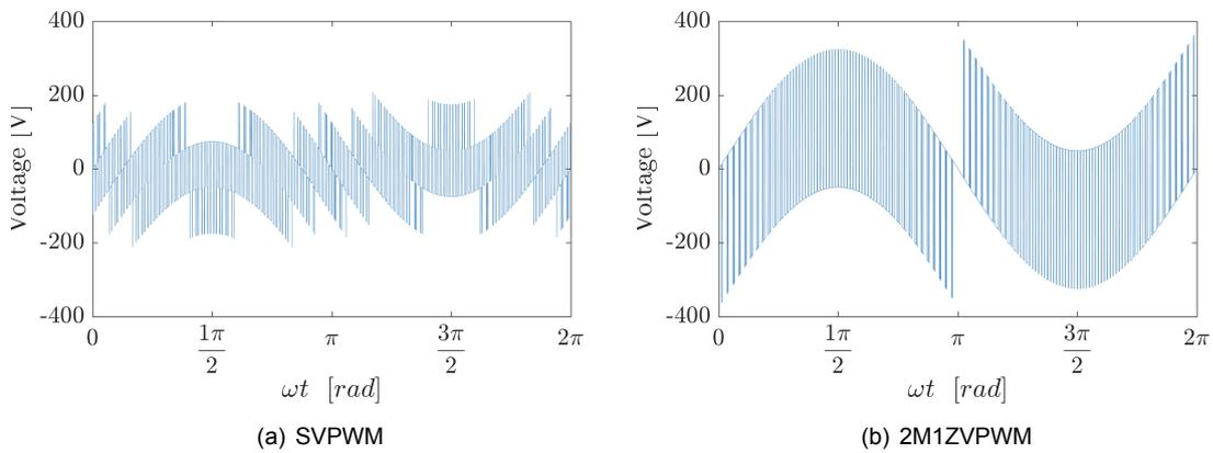
Figure E.7: Phase voltage ripple of the 3LNPC<sup>2</sup>.  $F_{sw} = 4kHz$
