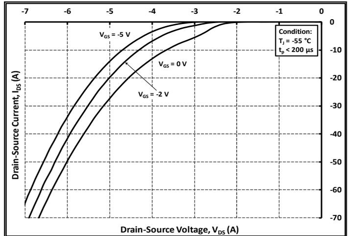
Figure 8. Body Diode Characteristic at  $-55\text{ }^\circ\text{C}$
