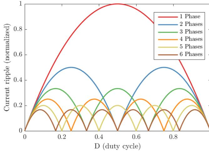
Figure 5.3: Input current ripple versus duty cycle for different levels of interleaving
