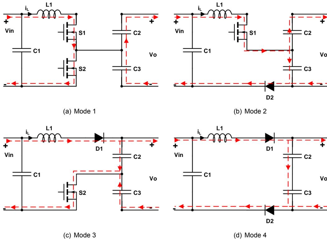
Figure 5.20: Switching states of the TLBC
