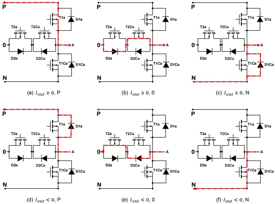
Figure 7.31: Switching states of the of the 3LT<sup>2</sup>C
