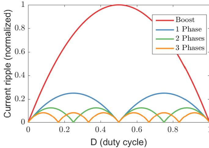
Figure 5.22: Input current ripple for the TLBC versus the normal boost converter
