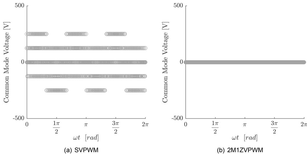
Figure 7.24: Common Mode Voltage of the 3LNPC<sup>2</sup>
