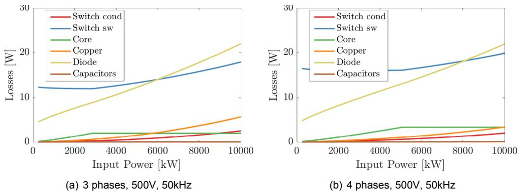
Figure 5.6: Losses versus input power for 3 and 4 phases at 500V
