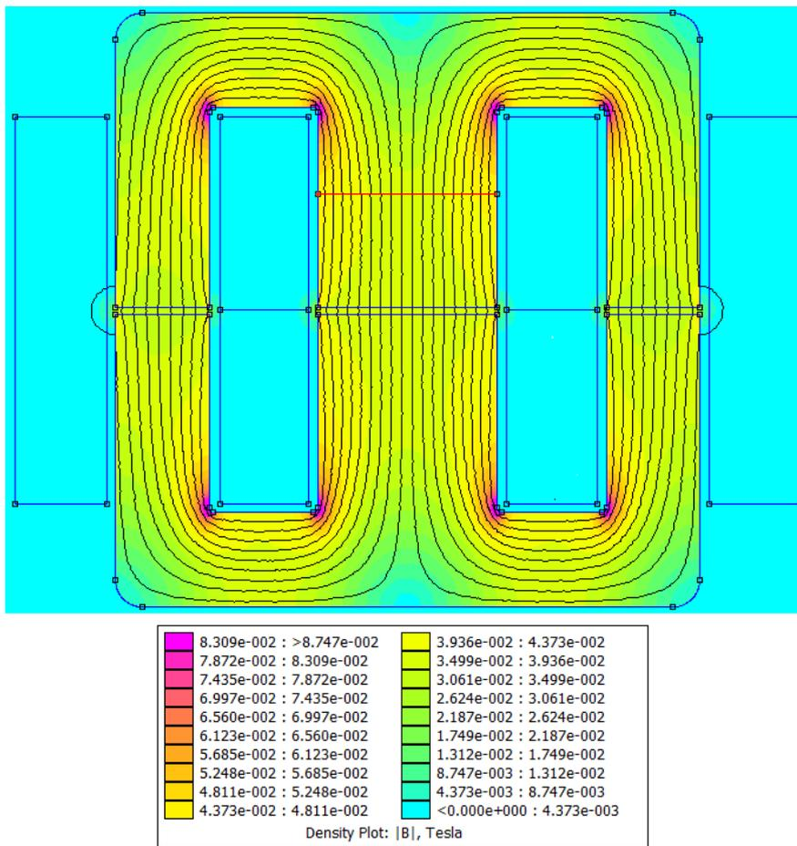
Figure B.2: FEM results of the 3 phases IBC inductor
