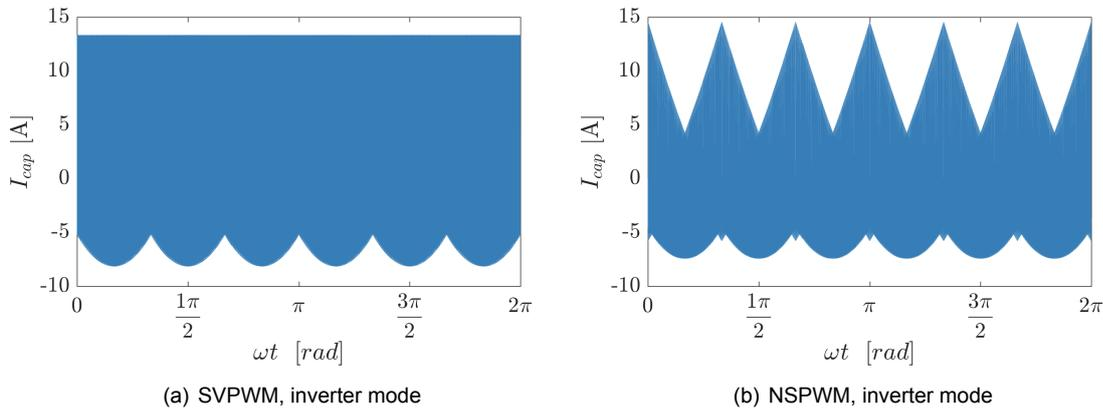
Figure 7.10: Input capacitor current of the 2LC,  $F_{sw} = 50$  kHz
