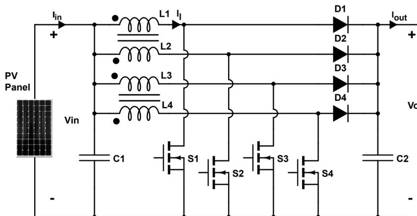
Figure 5.10: Structure of a four phases CIIBC
