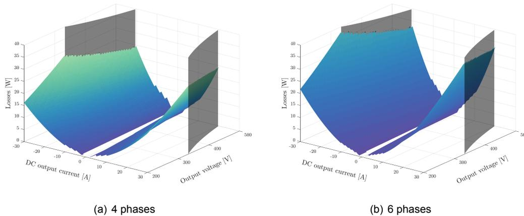
Figure 6.18: Losses in the magnetic elements of the IBFC
