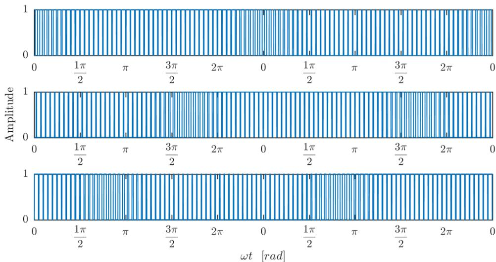
Figure E.1: Gate signals of the upper switches of the 2LC in SVPWM,  $F_{sw} = 4kHz$
