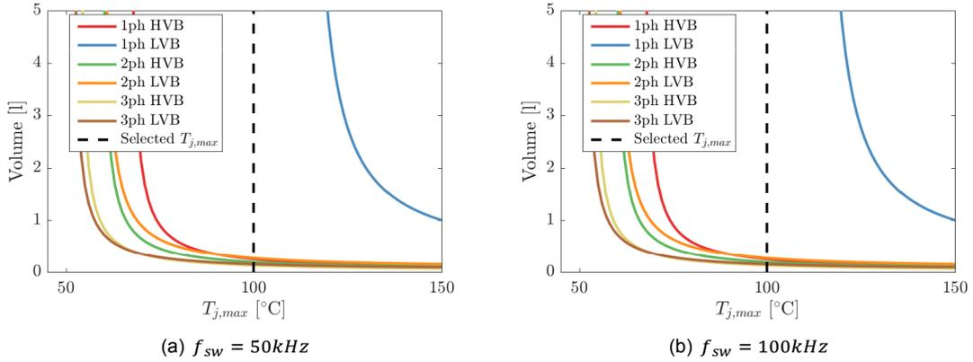
Figure 6.11: DAB cooling system size for different values of  $T_{j,max}$ .
