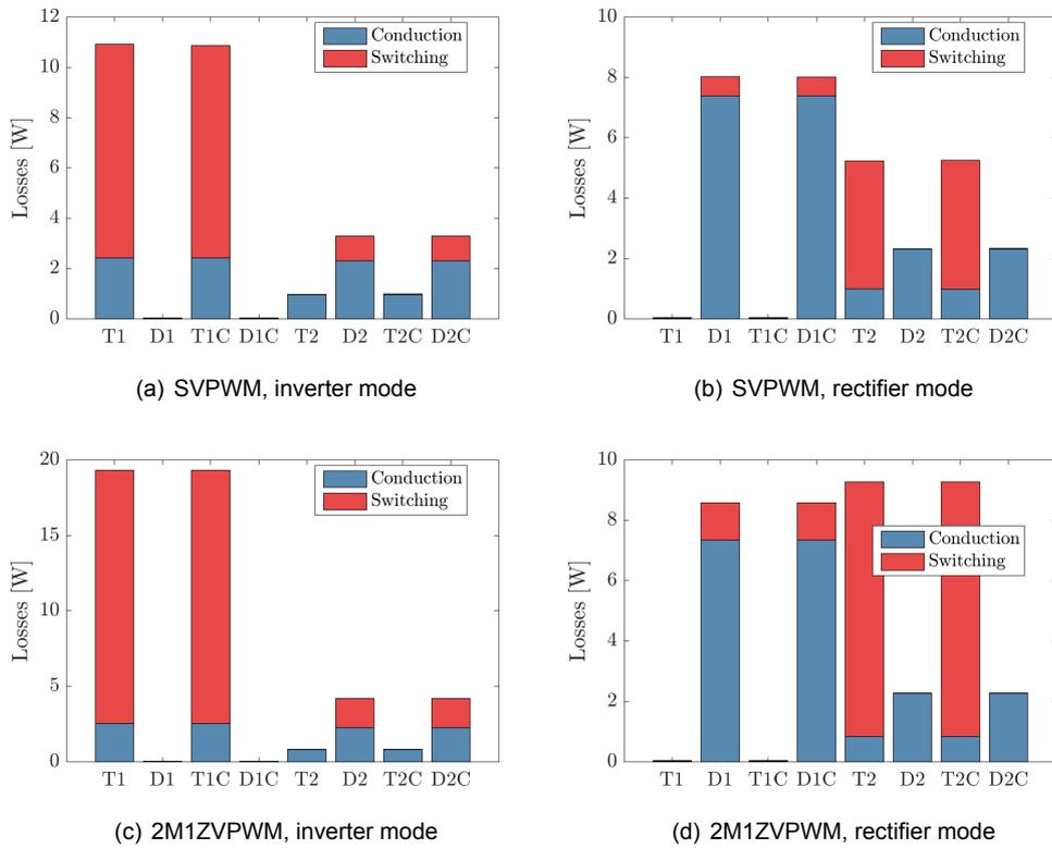
Figure 7.34: Losses of the 3LT<sup>2</sup>C,  $F_{sw} = 50$  kHz
