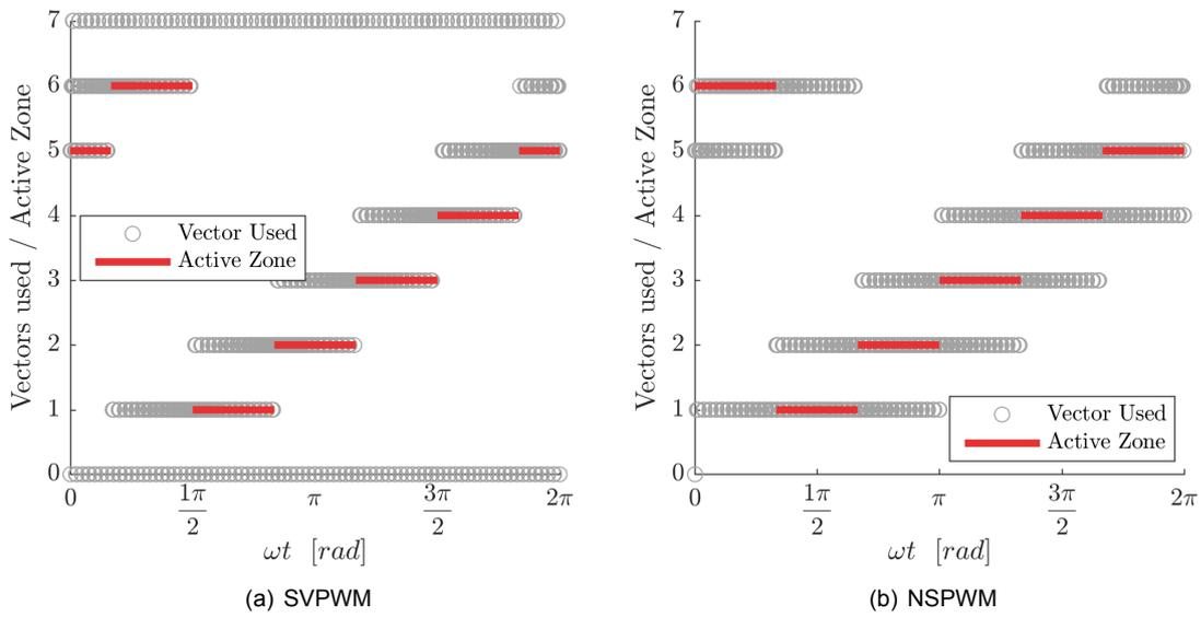
Figure E.3: Used vectors of the 2LC using SVPWM and NSPWM,  $F_{sw} = 4kHz$
