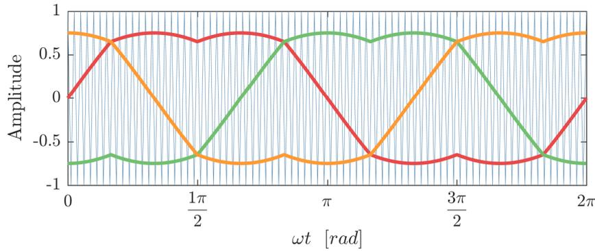
Figure 7.4: SVM like reference signal versus carrier signal
