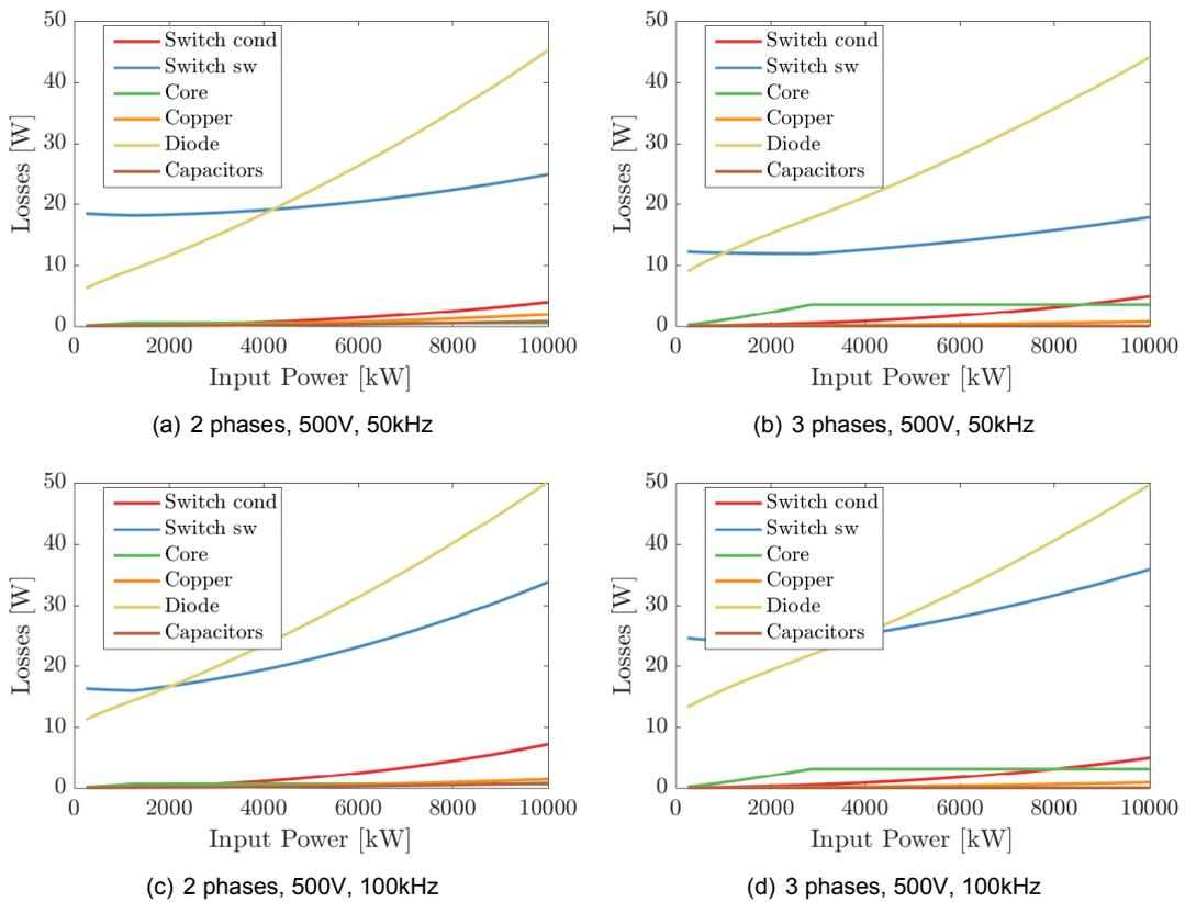
Figure 5.25: Losses versus input power for 3 and 4 phases at 500V
