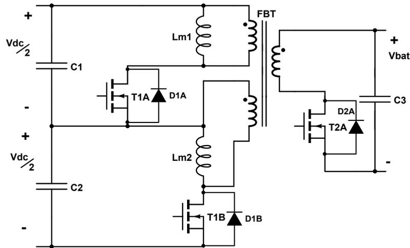
Figure 2.11: Structure of the IBFC
