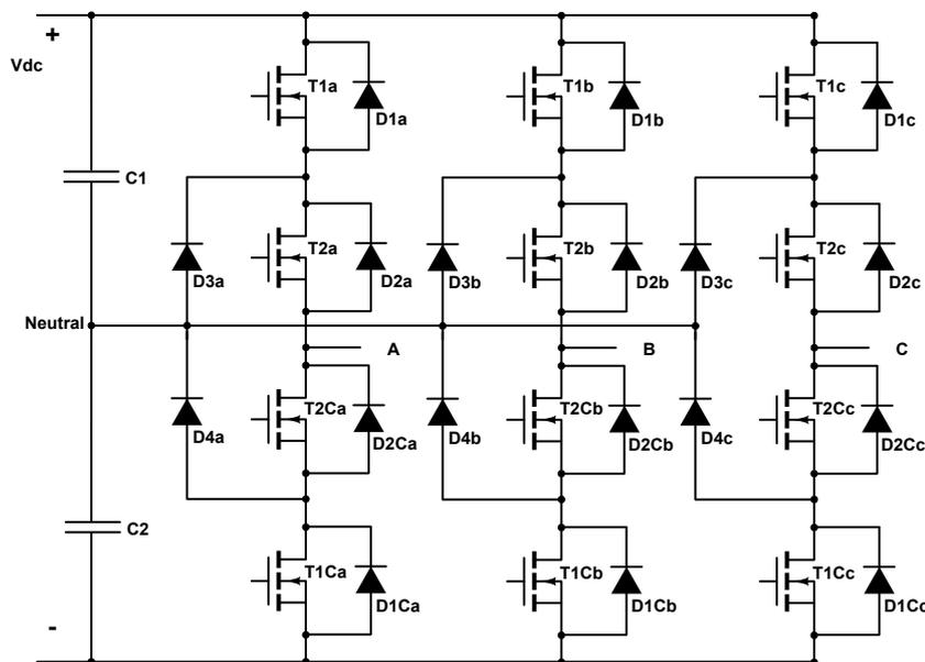
Figure 7.17: Structure of the 3LNPC<sup>2</sup>
