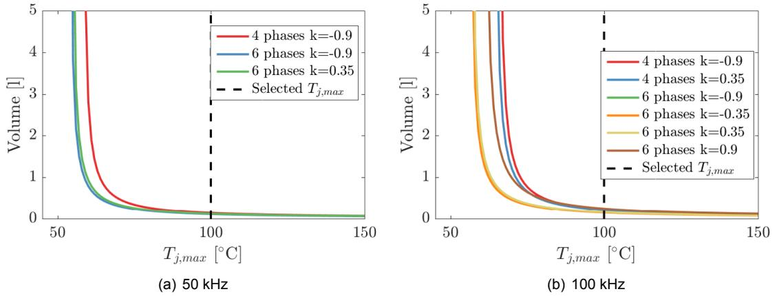
Figure 5.16: CIIBC cooling system size for different values of  $T_{j,max}$
