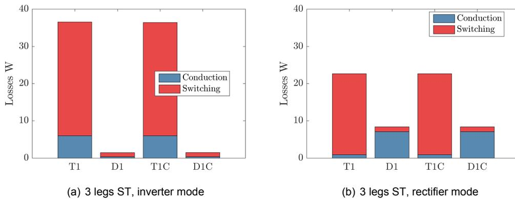
Figure 8.7: Losses of the qZSI,  $F_{sw} = 50$  kHz
