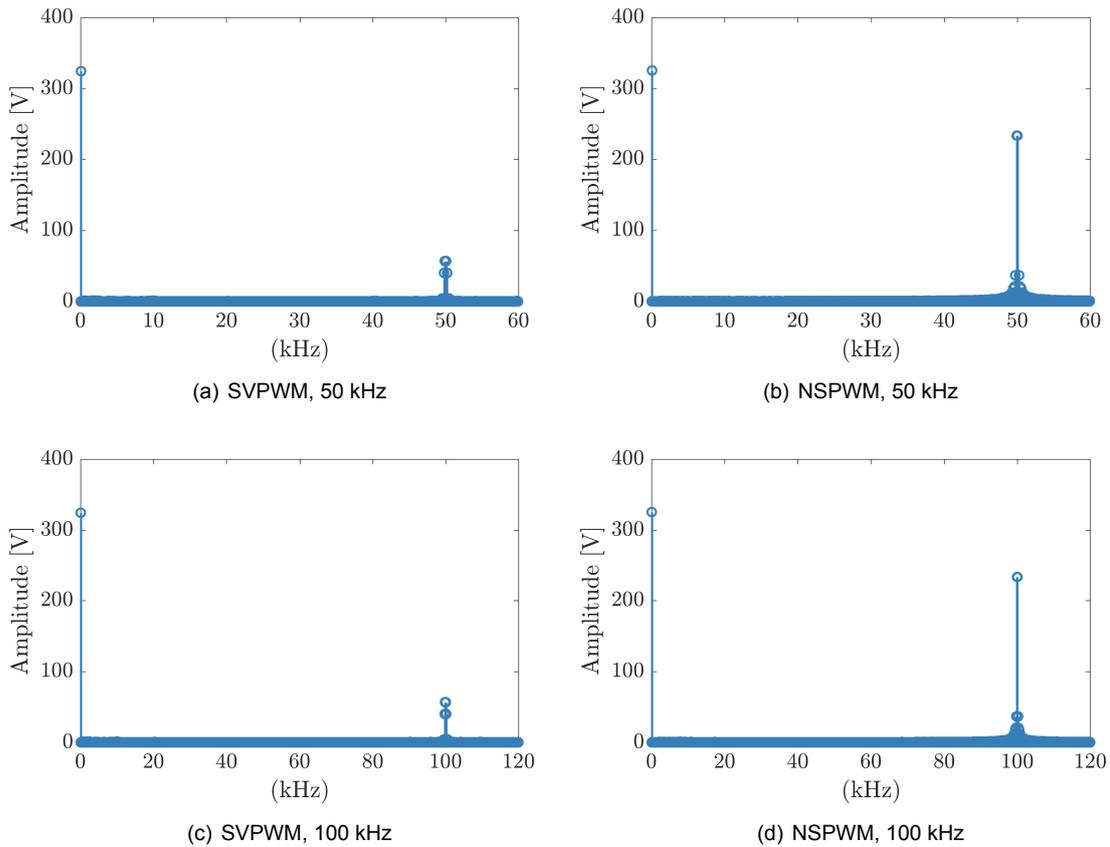
Figure 7.9: FFT of the 2LC for both modulation techniques.
