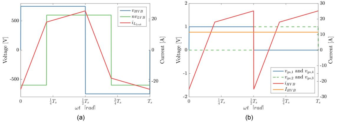
Figure 6.3: Operating waveforms of the DAB ( $V_{HVB} = 750$ ,  $V_{LVB} = 300$ ,  $T_\varphi = 0.2T_{sw}$ ,  $n = 2$ ).
