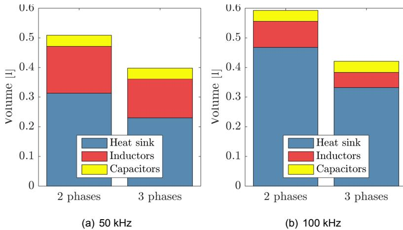
Figure 5.27: Volume of the different possible configurations of the IBC
