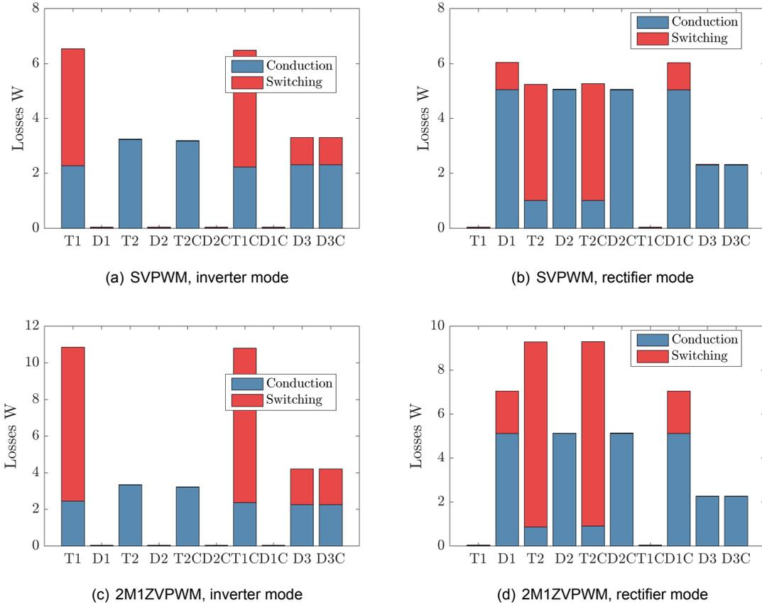
Figure 7.27: Losses of the 3LNPC<sup>2</sup>,  $F_{sw} = 50$  kHz
