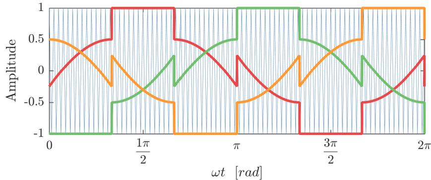
Figure 7.6: Reference waveforms and carrier signal of the NSPWM
