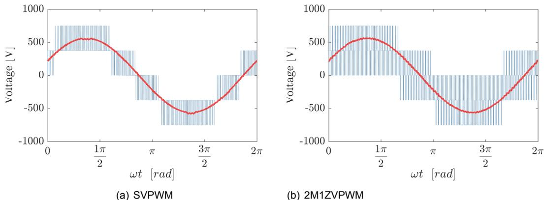
Figure E.5: Output line voltages of the 3LNPC<sup>2</sup> with both modulation techniques.  $F_{sw} = 4kHz$
