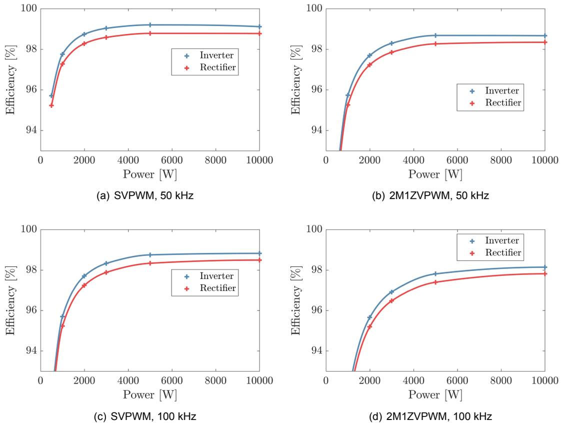
Figure 7.28: Efficiency of the 3LNPC<sup>2</sup> at different operating points.
