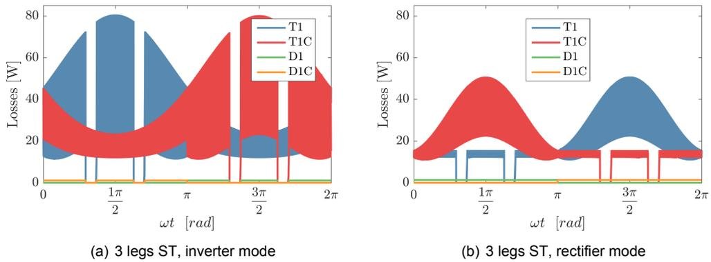
Figure 8.6: Switching losses of the qZSI,  $F_{sw} = 50$  kHz
