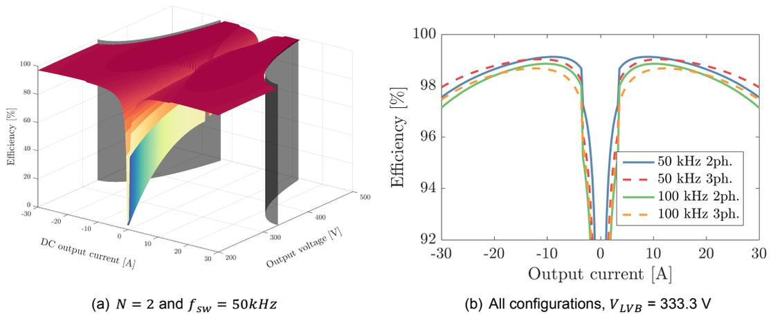
Figure 6.13: Efficiency of the DAB, 3D plot and all configurations
