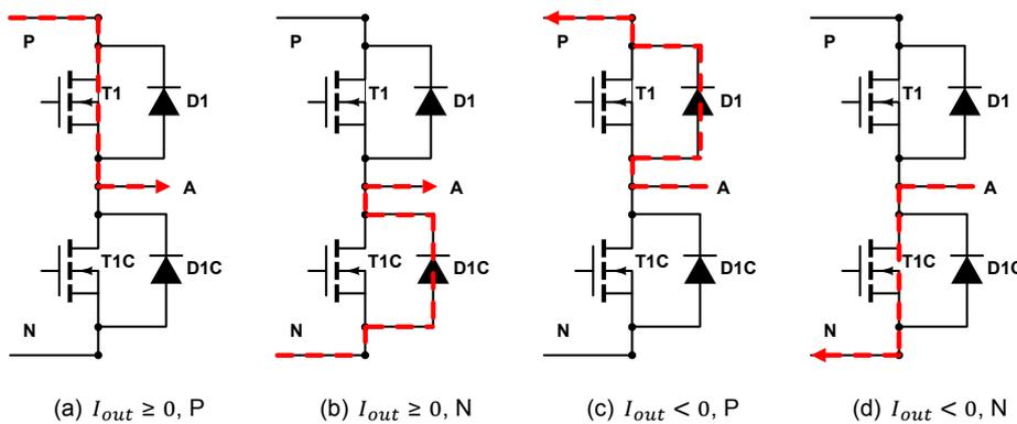
Figure 7.8: Switching states of the of the 2LC
