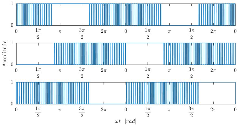
Figure E.2: Gate signals of the upper switches of the 2LC,  $F_{sw} = 4kHz$
