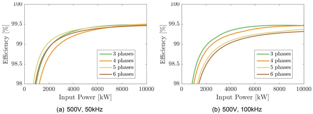
Figure 5.5: Efficiency versus input power for different levels of interleaving
