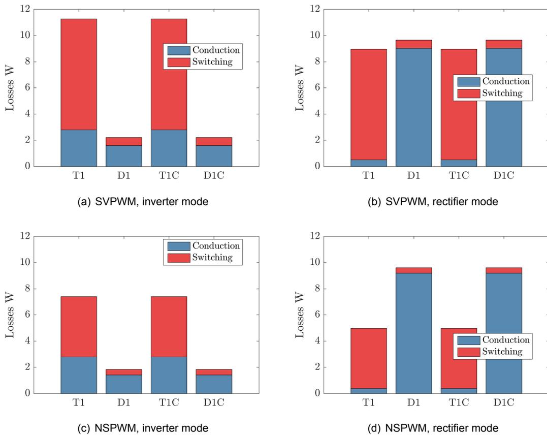
Figure 7.14: Losses of the 2LC,  $F_{sw} = 50$  kHz
