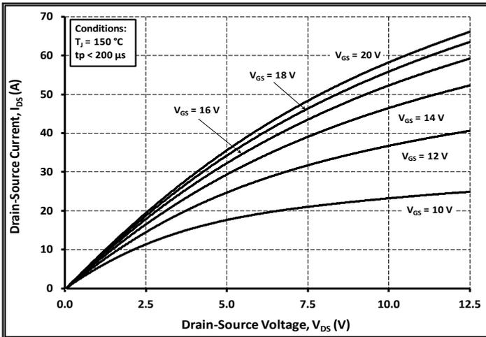
Figure 3. Output Characteristics  $T_J = 150\text{ }^\circ\text{C}$
