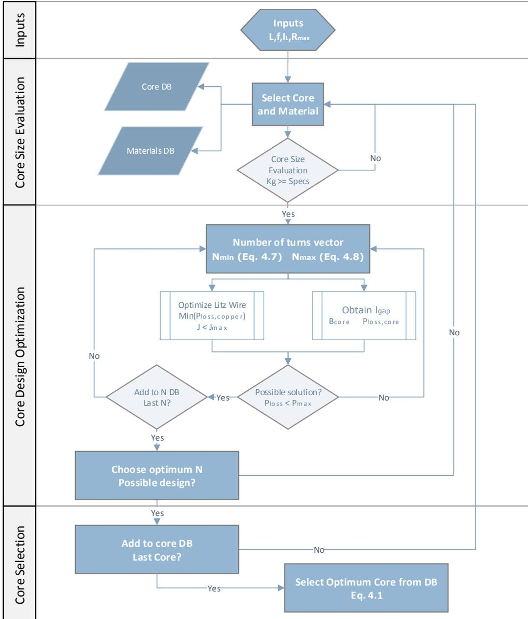
Figure 4.1: Flowchart of the power inductor design.
