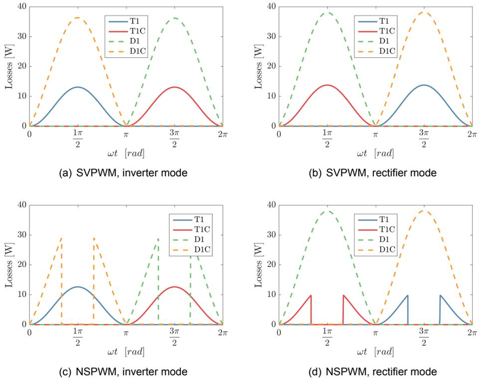
Figure 7.12: Conduction losses of the 2LC,  $F_{sw} = 50$  kHz
