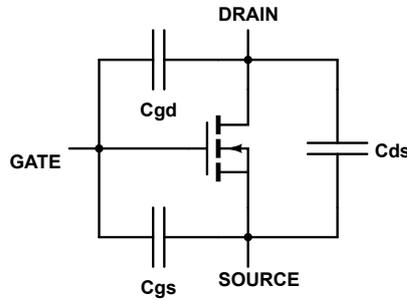
Figure 3.2: Power mosfet parasitic capacitances
