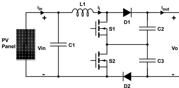
Fig. 8: Structure of a one phase TLBC
