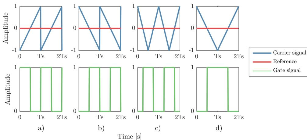
Figure 7.7: Different triangular waves and resulting gate signals
