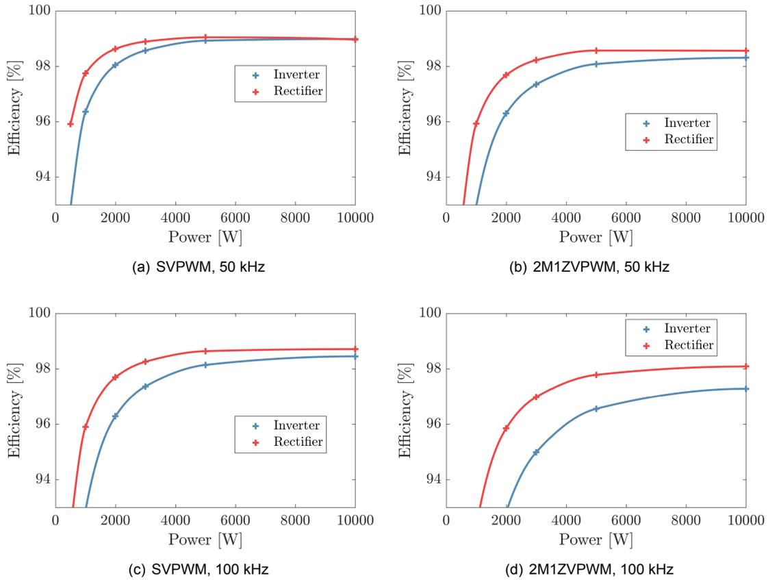
Figure 7.35: Efficiency of the 3LT<sup>2</sup>C at different operating points.
