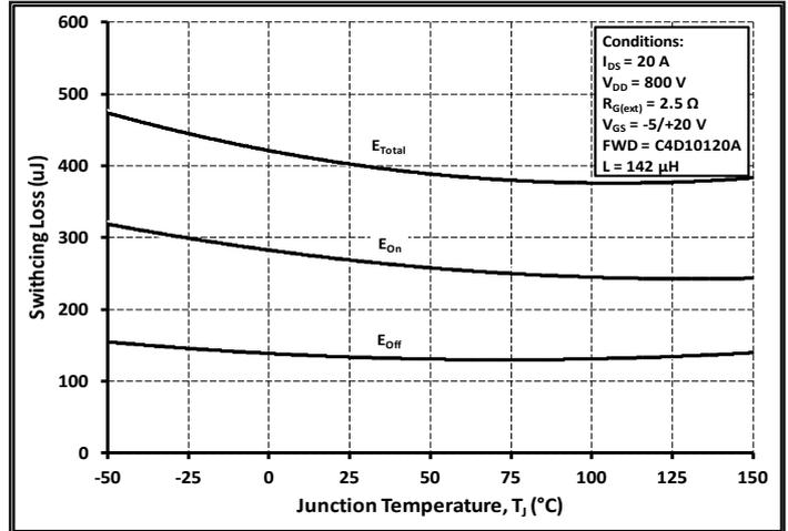
Figure 26. Clamped Inductive Switching Energy vs. Temperature
