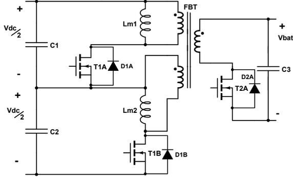
Fig. 12: Structure of the IBFC
