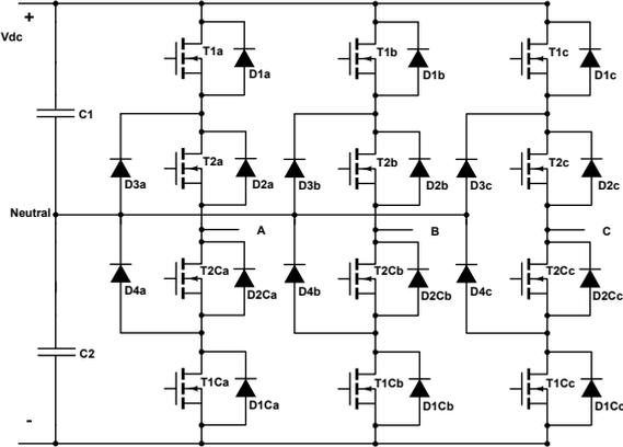
Fig. 16: Structure of the 3LNPC
