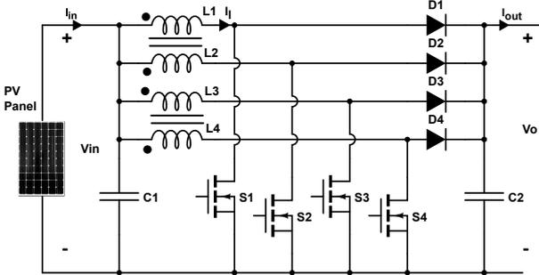
Fig. 7: Structure of a four phases CIIBC
