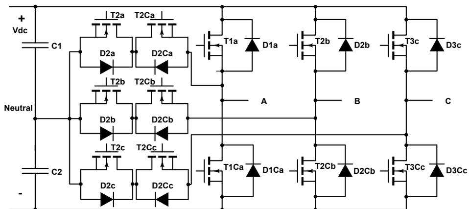
Figure 2.14: Structure of the 3LT<sup>2</sup>C
