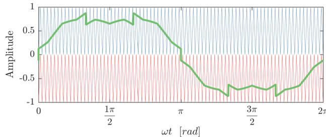
Figure 7.19: SVM like reference signal versus carrier signal
