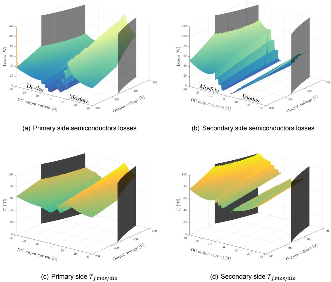
Figure 6.19: Semiconductor losses and temperatures of the IBFC, 4 phases
