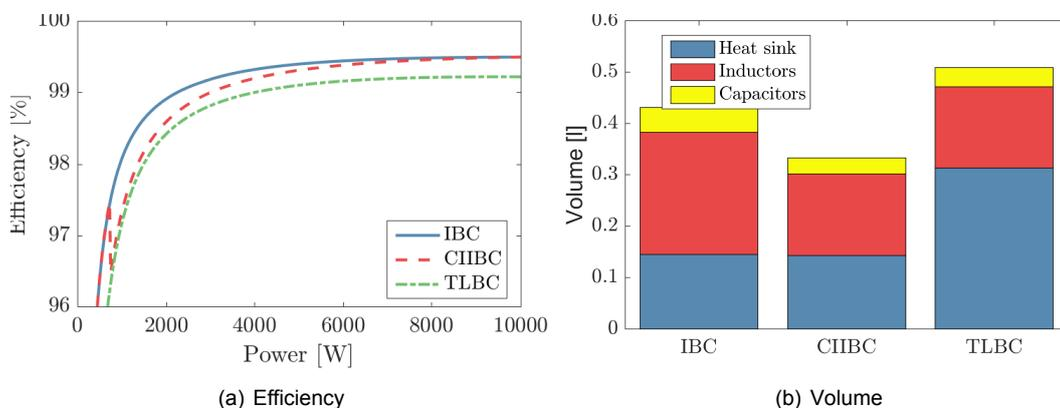
Figure 5.28: Results of the optimal topologies configurations of the PV port.
