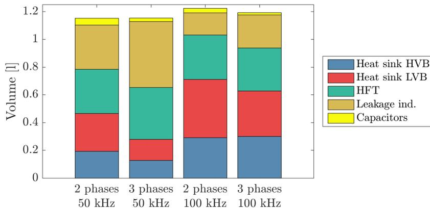
Figure 6.12: Distribution of the total volume of the different DAB configurations
