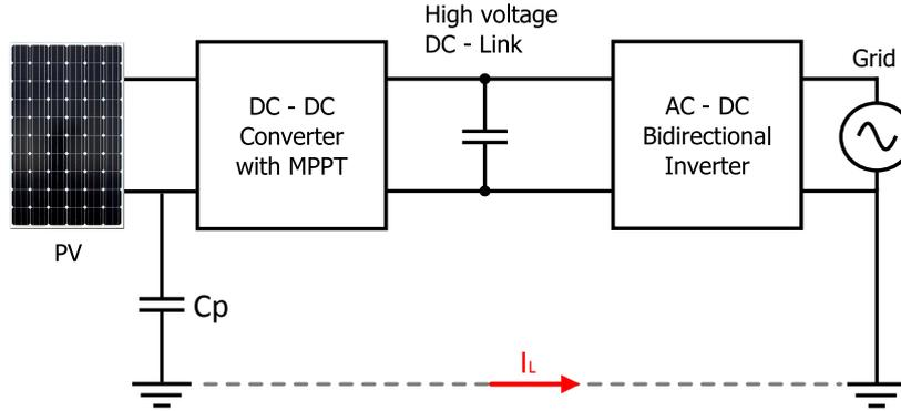
Figure 2.17: Leakage current due to parasitic capacitance in PV systems.
