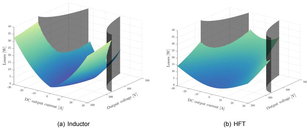
Figure 6.8: Losses at the magnetic elements of the DAB,  $N = 2$  and  $f_{sw} = 50kHz$
