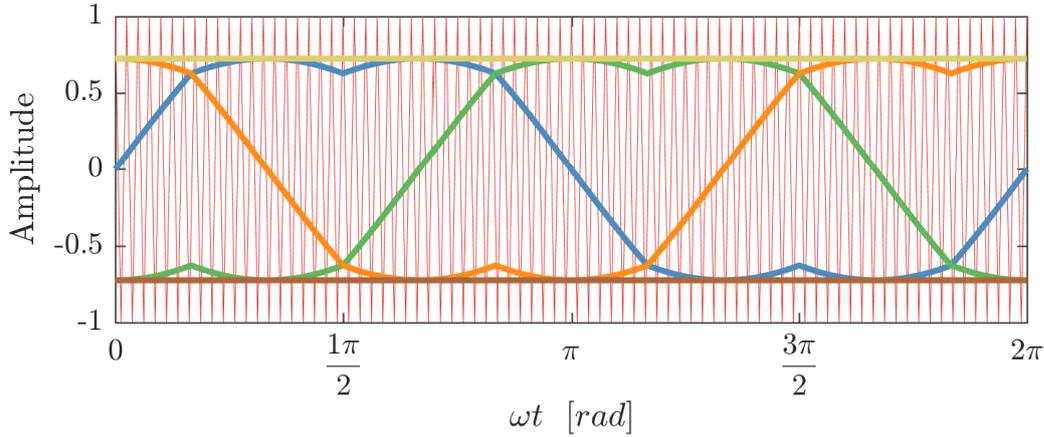
Figure 8.3: Reference waveforms versus triangular wave in qZSI ( $V_{in} = 350V$ )
