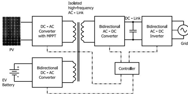
Fig. 4: Block diagram of a three-port converter with an inner AC link.
