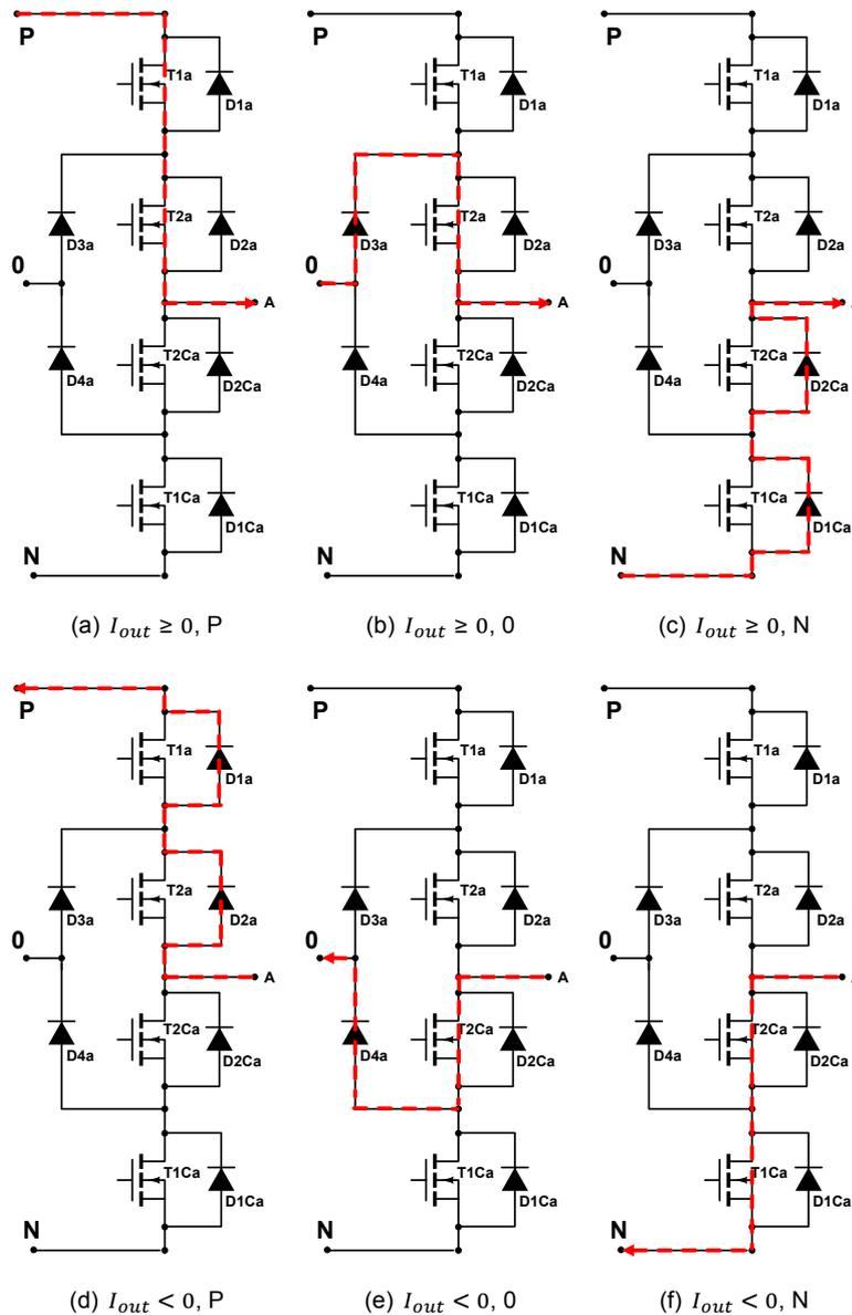
Figure 7.22: Switching states of the of the 3LNPC<sup>2</sup>
