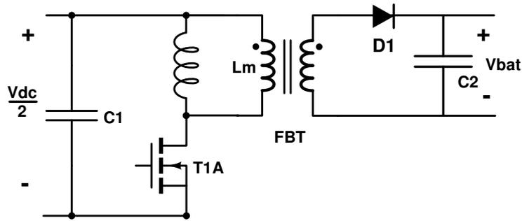
Figure 2.10: Structure of the Flyback converter.
