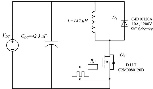
Figure 30. Clamped Inductive Switching Waveform Test Circuit
