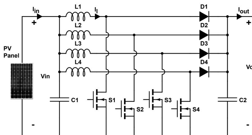
Figure 5.1: Structure of a four phases IBC
