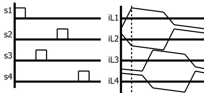
Figure D.2: Switching patterns and inductor current ripple in the CIIBC.
