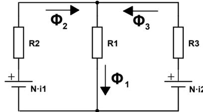
Figure 4.2: Magnetic model of the coupled inductor with the coils in the outer legs.
