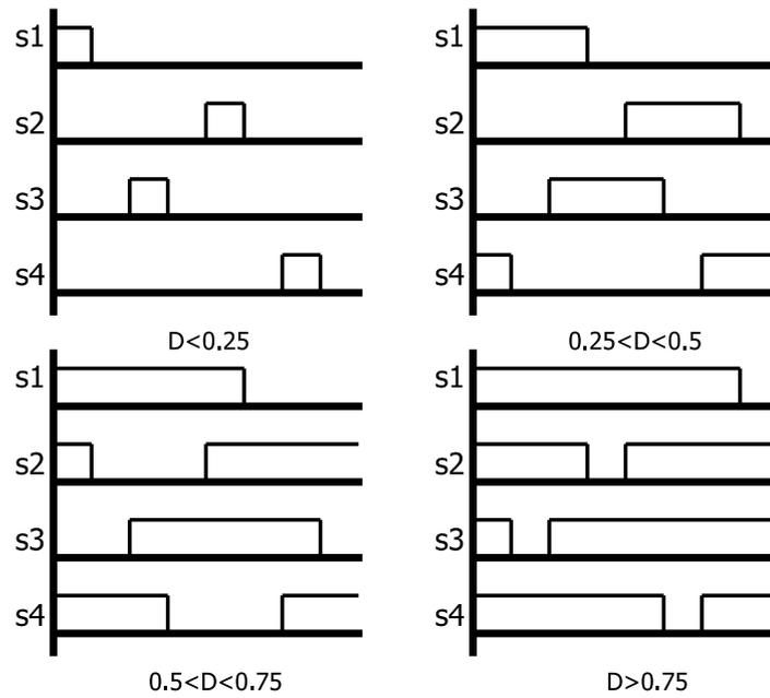
Figure D.1: Switching patterns for different values of duty cycle in the CIIBC.
