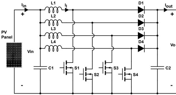
Fig. 6: Structure of a four phases IBC
