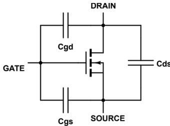
Fig. 5: Power mosfet parasitic capacitances
