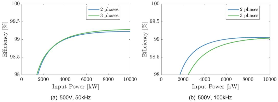
Figure 5.24: Efficiency versus input power for different levels of interleaving
