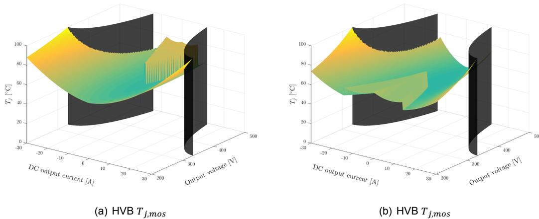
Figure 6.10: Semicondutor temperatures of the DAB,  $N = 2$  and  $f_{sw} = 50kHz$
