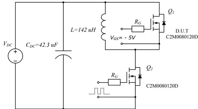
Figure 31. Body Diode Recovery Test Circuit
