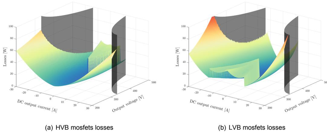
Figure 6.9: Semicondutor losses of the DAB,  $N = 2$  and  $f_{sw} = 50kHz$
