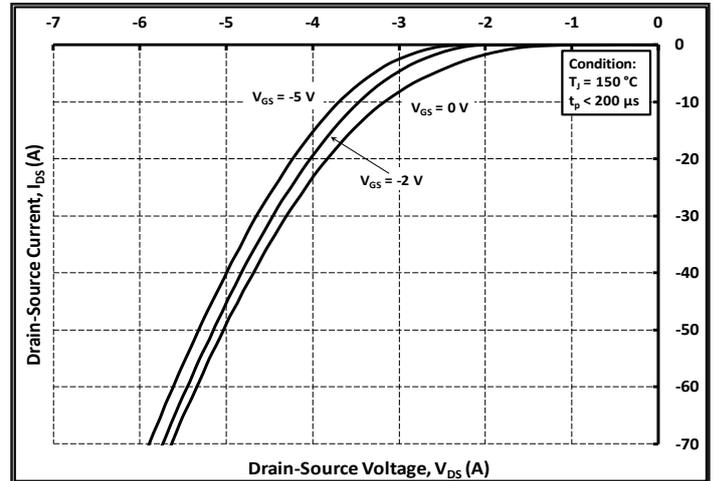
Figure 10. Body Diode Characteristic at  $150\text{ }^\circ\text{C}$
