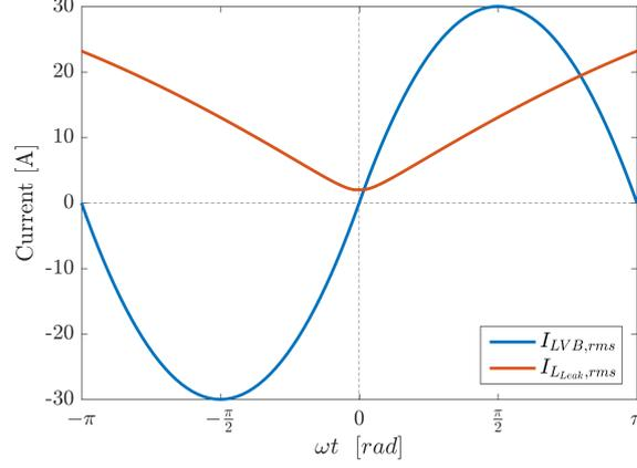
Figure 6.4: Main currents of the DAB ( $V_1 = 750V$ ,  $V_2 = 333.33V$ ,  $T_\varphi = 0.25T_{sw}$ ,  $n = 2$ )
