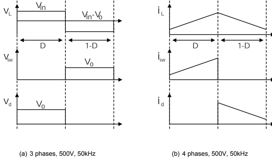
Figure 5.2: Voltage and current waveforms of the IBC in CICM
