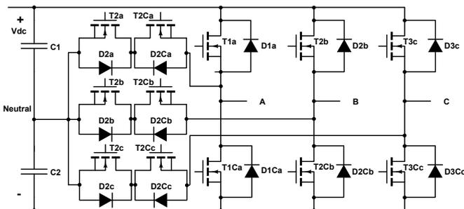
Fig. 17: Structure of the 3LTC
