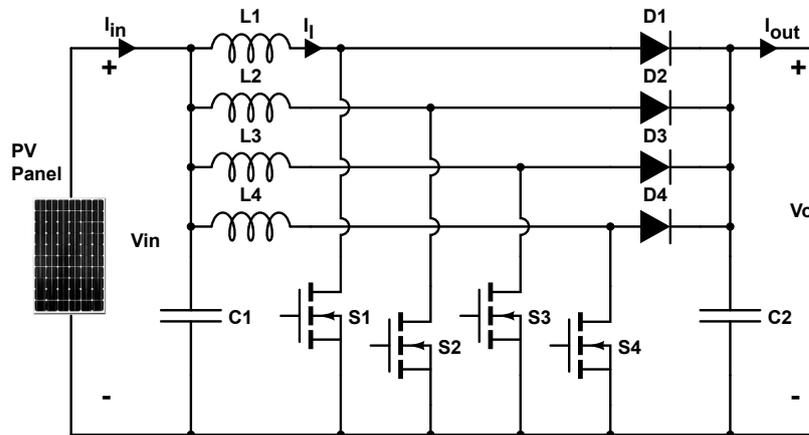
Figure 2.6: Structure of a four phases IBC
