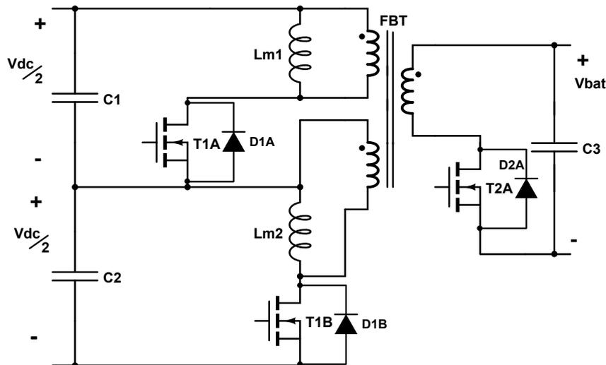
Figure 6.14: Structure of a one phase IBFC
