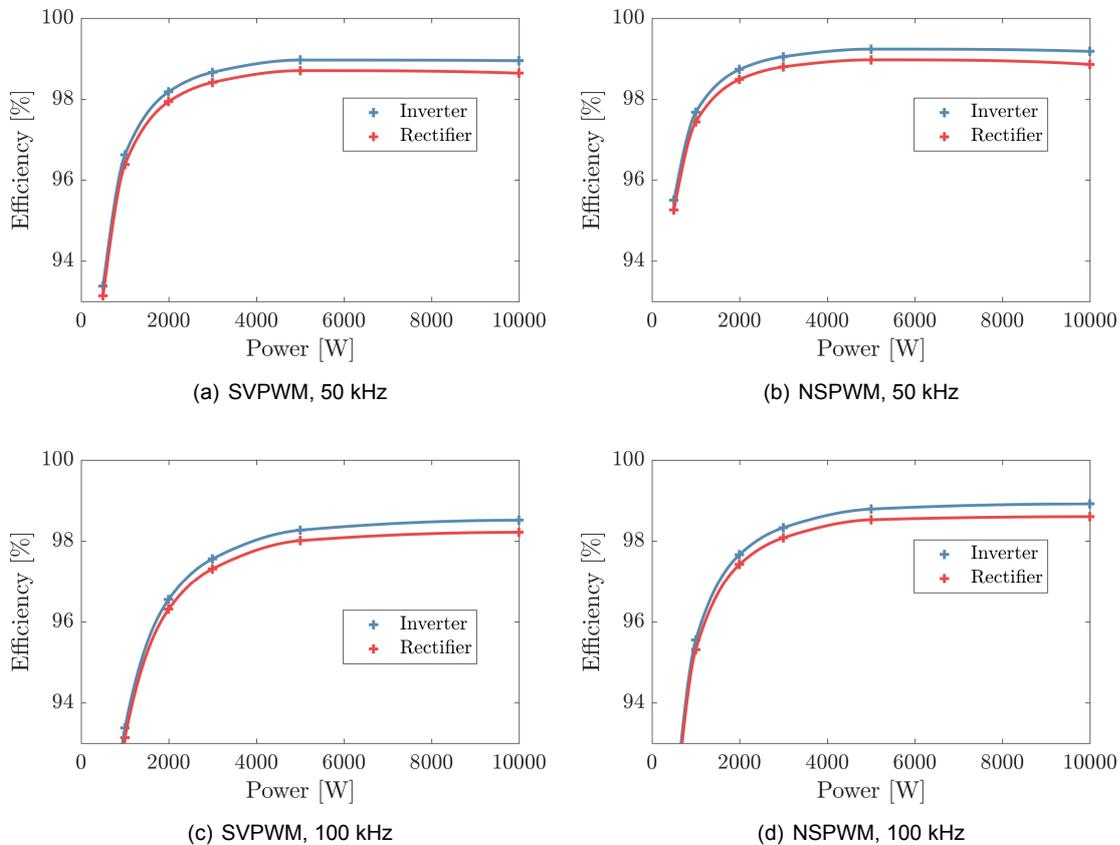
Figure 7.15: Efficiency of the 2LC at different operating points
