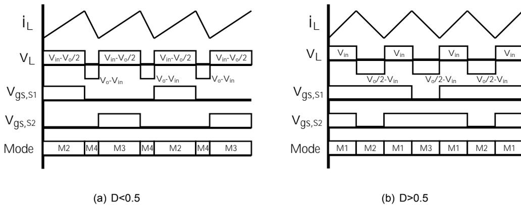
Figure 5.21: Waveforms of the TLBC for different duty cycles, CICM
