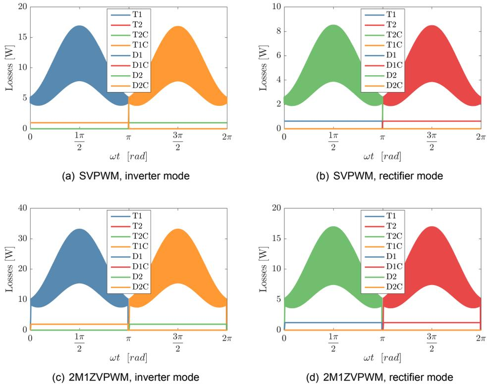
Figure 7.33: Switching losses of the 3LT<sup>2</sup>C,  $F_{sw} = 50$  kHz
