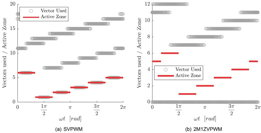
Figure E.6: Used vectors of the 3LNPC<sup>2</sup> using SVPWM and 2M1ZVPWM.  $F_{sw} = 4kHz$
