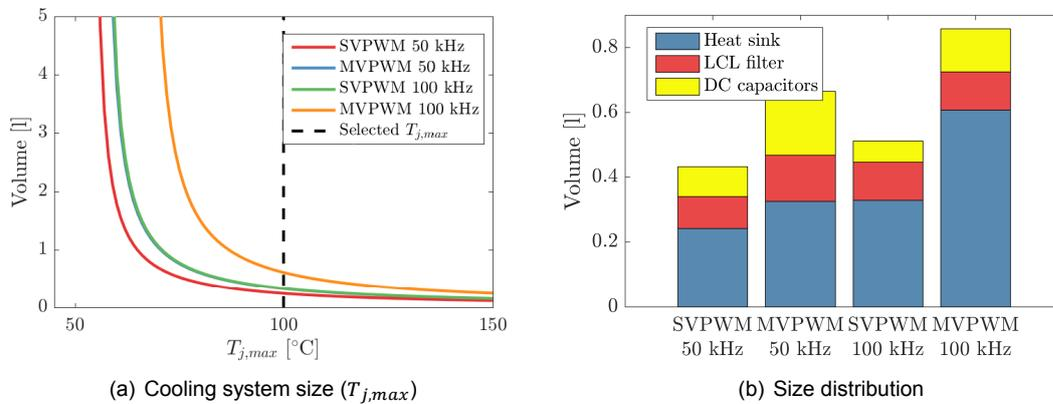
Figure 7.29: 3LNPC<sup>2</sup> system size
