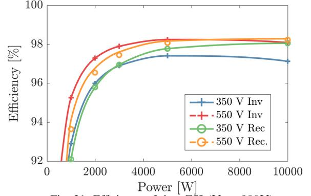
Fig. 21: Efficiency of the qZSI ( $V_p = 230$ V)
