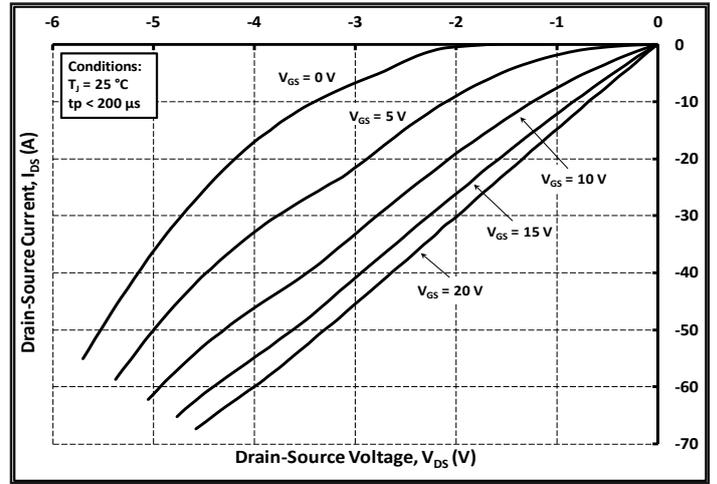
Figure 14. 3rd Quadrant Characteristic at  $25\text{ }^\circ\text{C}$
