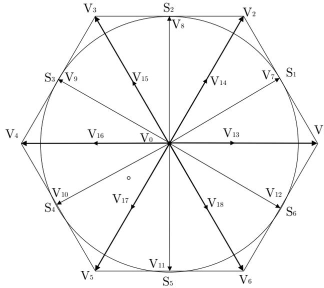
Figure 7.18: Working principle of the SVM.
