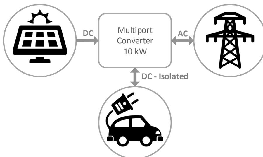
Figure 2.1: Block diagram of three-port DC-DC-AC converter
