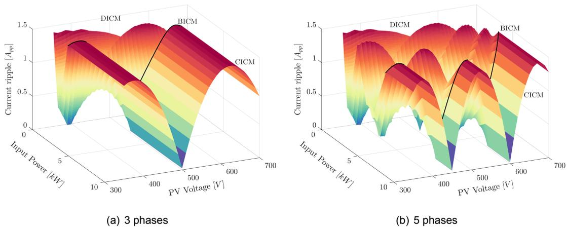
Figure 5.4: Input current ripple versus input voltage and power for different levels of interleaving
