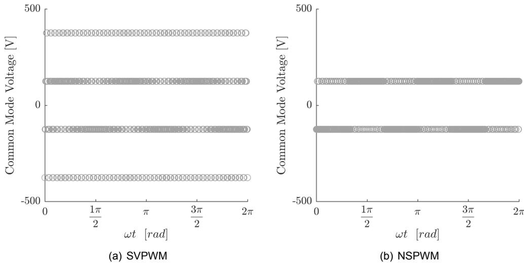
Figure 7.11: Common Mode Voltage of the 2LC
