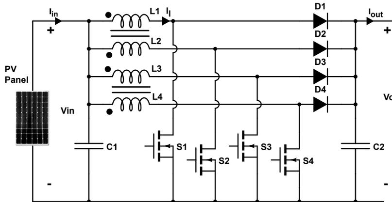
Figure 2.7: Structure of a four phases CIIBC
