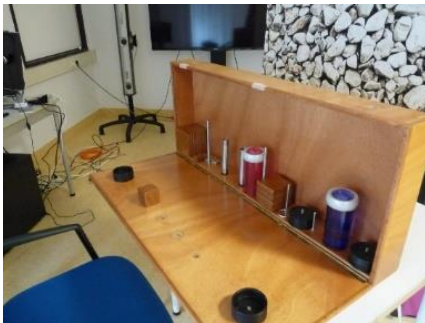
Fig. 4. The ARAT kit used for reach and grasp movements in real world.
