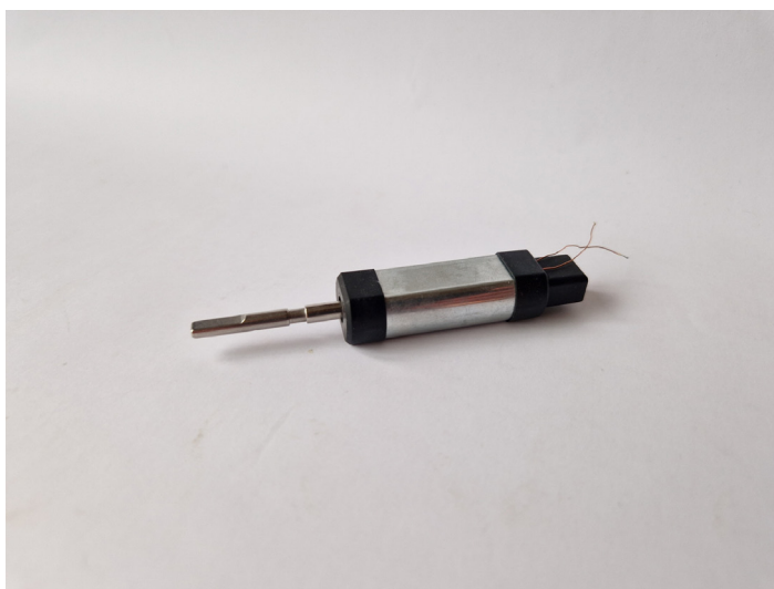
Figure 22: Boombrush motor. The brush axis is fixed directly in the motor.
