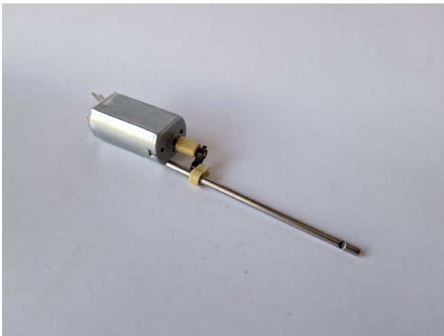
Figure 28: The 2D rotating brush technology, from the motor to the brush axis.
