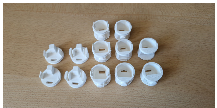
Figure 55: 3d printed test models of the snap-fit style release button on the bottom cap.
