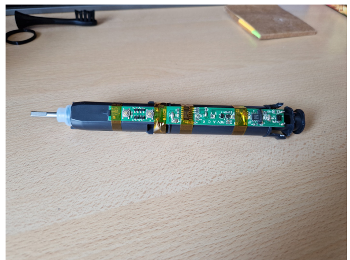
Figure 25: The four tapes that have to be removed prior to accessing the electronics of the Boombrush.
