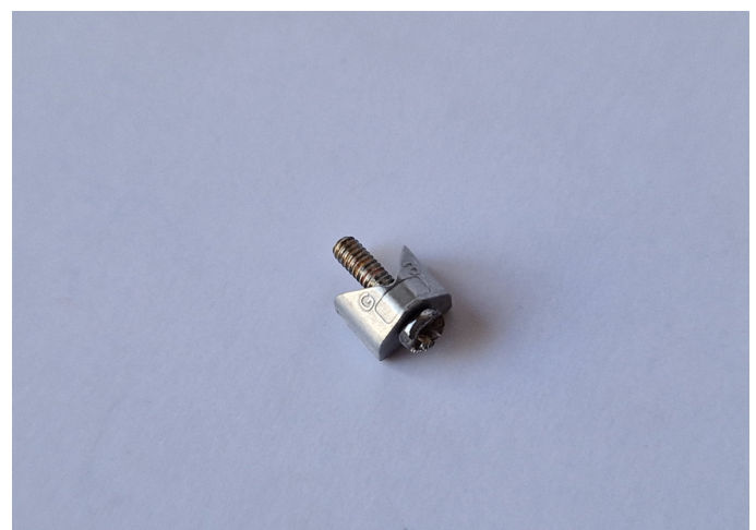
Figure 44: The screw used in the magnet lock of the Philips Sonicare Easyclean is fixed using Loctite. To apply enough force to remove the screw, the screw had to be destroyed.
