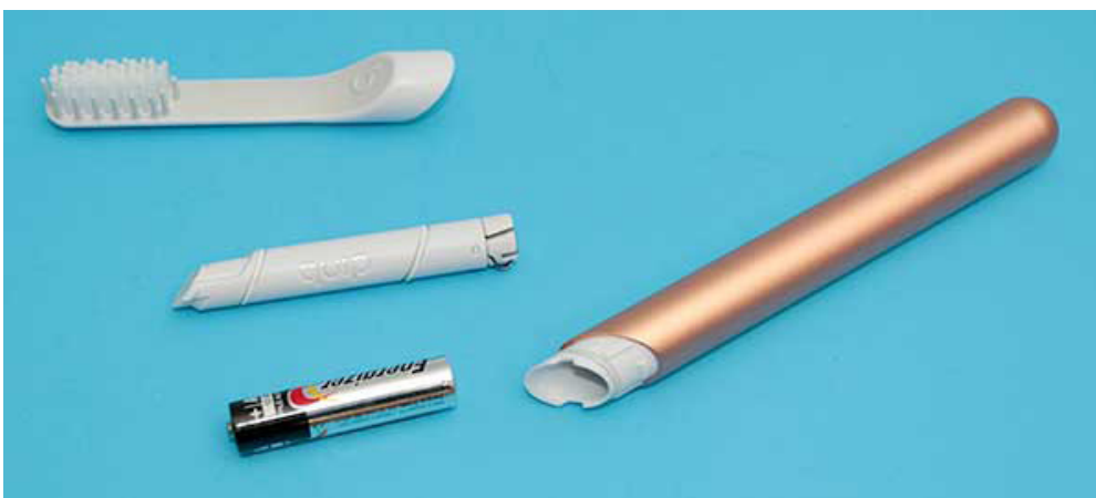
Figure 8: Quip Adult electric toothbrush with its AAA battery removed (Strietelmeier, 2017).
