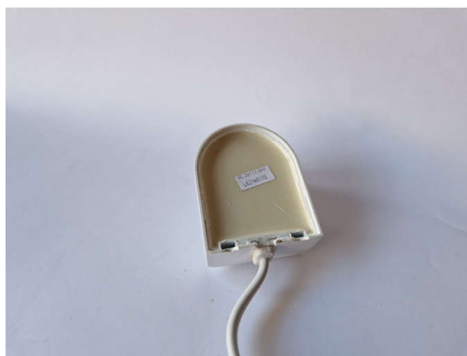
Figure 46: The charger of the Philips Sonicare Easyclean is filled, making the separation of electronics impossible.
