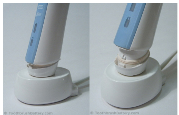
Figure 37: Removing the bottom cap with the charger (Toothbrushbattery.com, n.d.-b).
