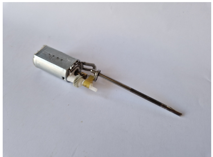
Figure 34: The 3D rotating brush technology, from the motor to the brush axis.
