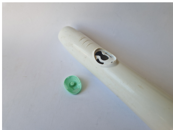
Figure 45: The power button of the Philips Sonicare Easyclean is an elastomer part with snapfits.
