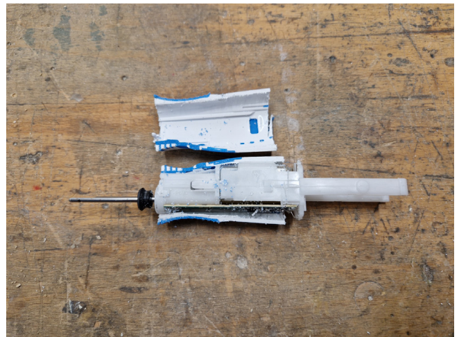
Figure 29: The Oral-B Advance Power was sawn open for complete disassembly.
