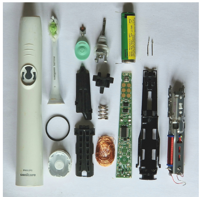
Figure 6: A disassembled Philips Sonicare Easyclean electric toothbrush.
