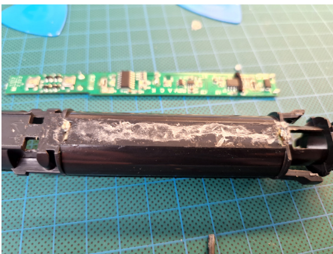
Figure 24: Boombrush uses glue to fix the PCB to the internal carriage.
