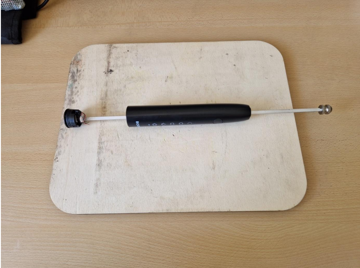
Figure 1: Boombrush modified for force testing.
