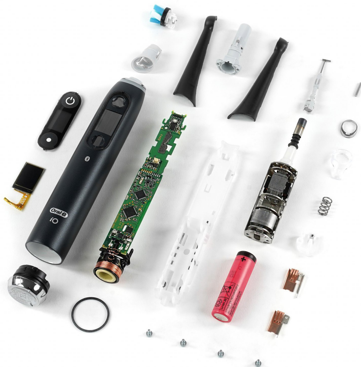
Figure 2: Disassembled Oral-B iO electric toothbrush (Isakeit, 2020).
