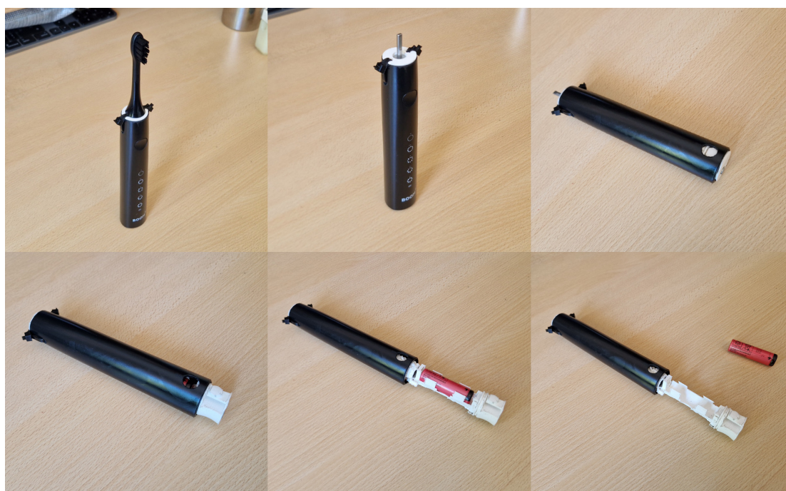
Figure 63: Prototype for the battery replacement procedure.
