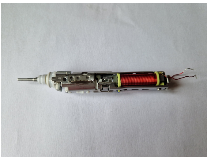
Figure 42: Brush mechanism of the Philips Sonicare Easyclean.
