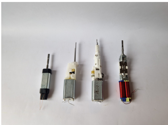
Figure 49: Overview of the four analysed brushes' brush technologies. From left to right: Boombbrush (sonic), Oral-B Advance Power (2d rotating), Oral-B Professional Clean (3d rotating), Philips Sonicare Easyclean (sonic).
