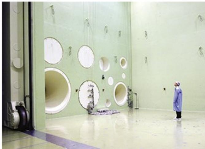
Figure 1.1: ESA's Large European Acoustic Facility. Photo: ESA
