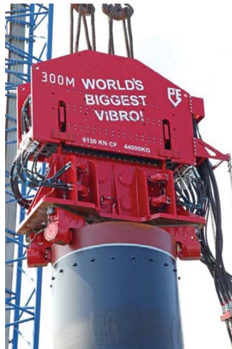
Figure 2.7: PVE 300M Vibratory hammer clamped directly to a monopile.
