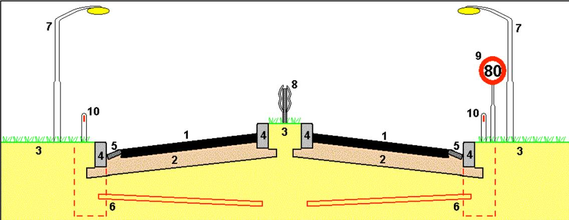
Figure 1 :Composition of road structure
