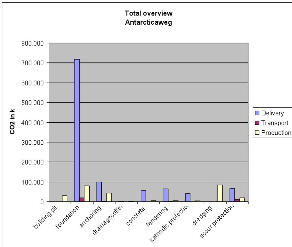
Figure 6 Carbon footprint for Antarticaweg quay wall in more detail
