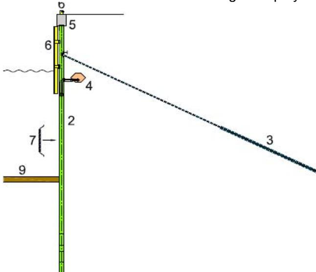
Figure 2: Anchored sheet pile wall quay wall
