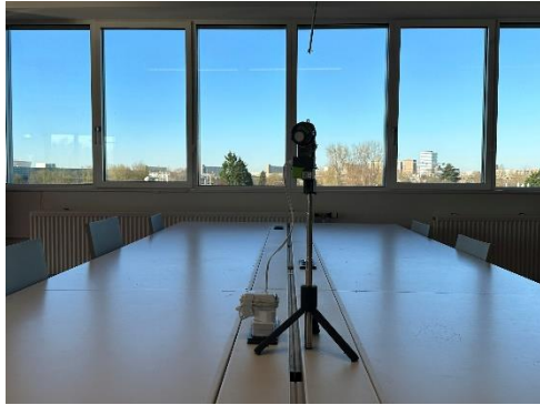
Figure 32: CozIR and Sensirion SPS30 on desk level
