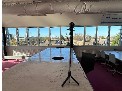
Figure 33: CozIR on room level
