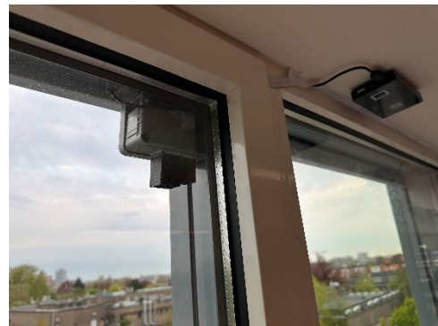
Figure 37: Outdoor placement of Sensirion SEN54
