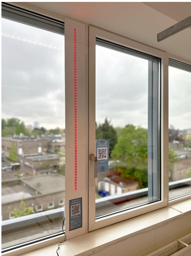
Figure 40: Window feedback system that was built and implemented inside the BT-studio
