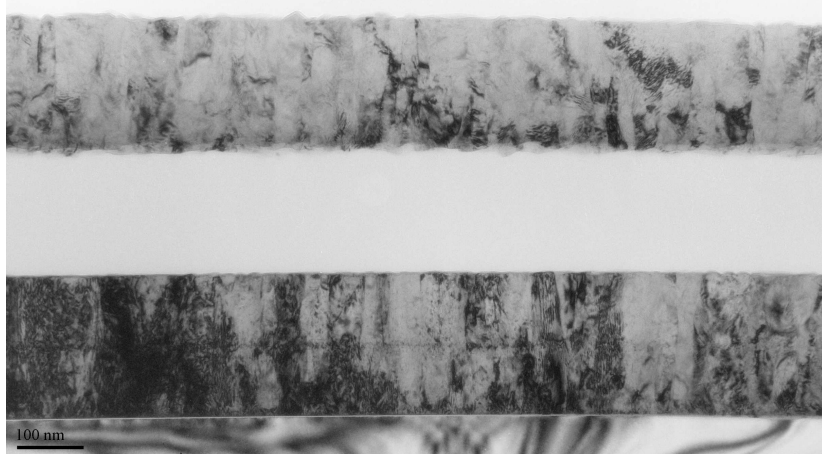
Figure 4.4: Bright field transmission electron micrograph [13] of a heterostructure of niobium, silicon dioxide, and niobium, on top of a (111) silicon substrate. This structure is the same as the microstripline that is being used in this work.
