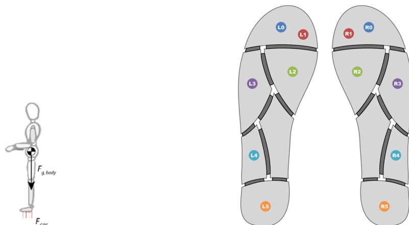
Figure 54 - Colour coded sensor map on the insole, six-sensor layout.
