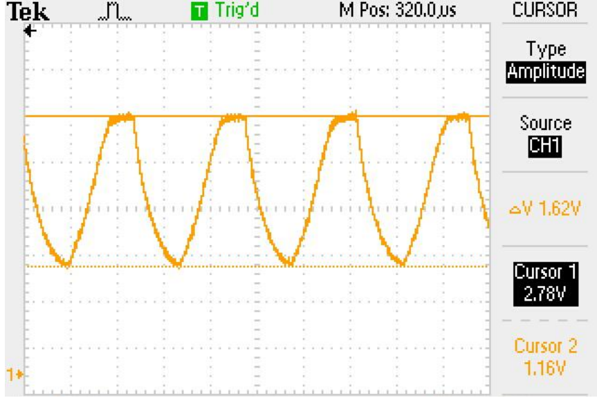
Figure 4.3: Two photodiodes shared amplifier structure readout with strong light intensity( TG1 = high ; TG2 = high )
