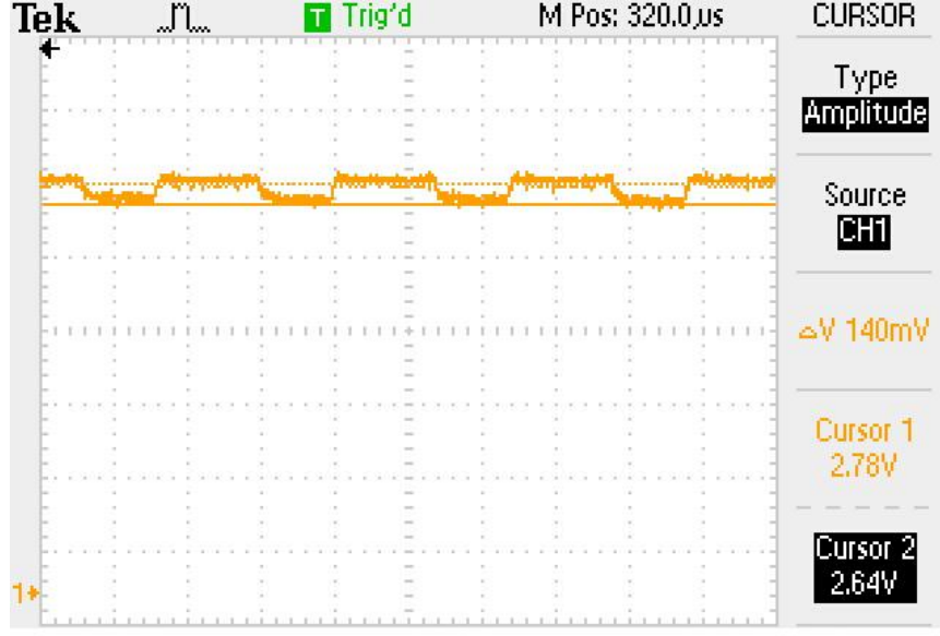
Figure 4.4: Two photodiodes shared amplifier structure readout with low light intensity( TG1 = high; TG2 = high )
