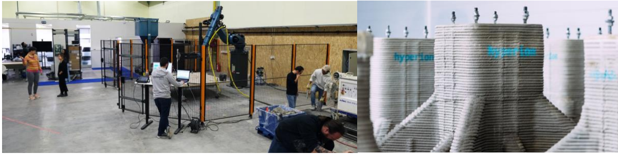
Figure 2: 3DCP Workspace in Espoo, Finland (left) and Infrastructure Foundation Products (right). Image courtesy of Hyperion Robotics (2022, 2025).
