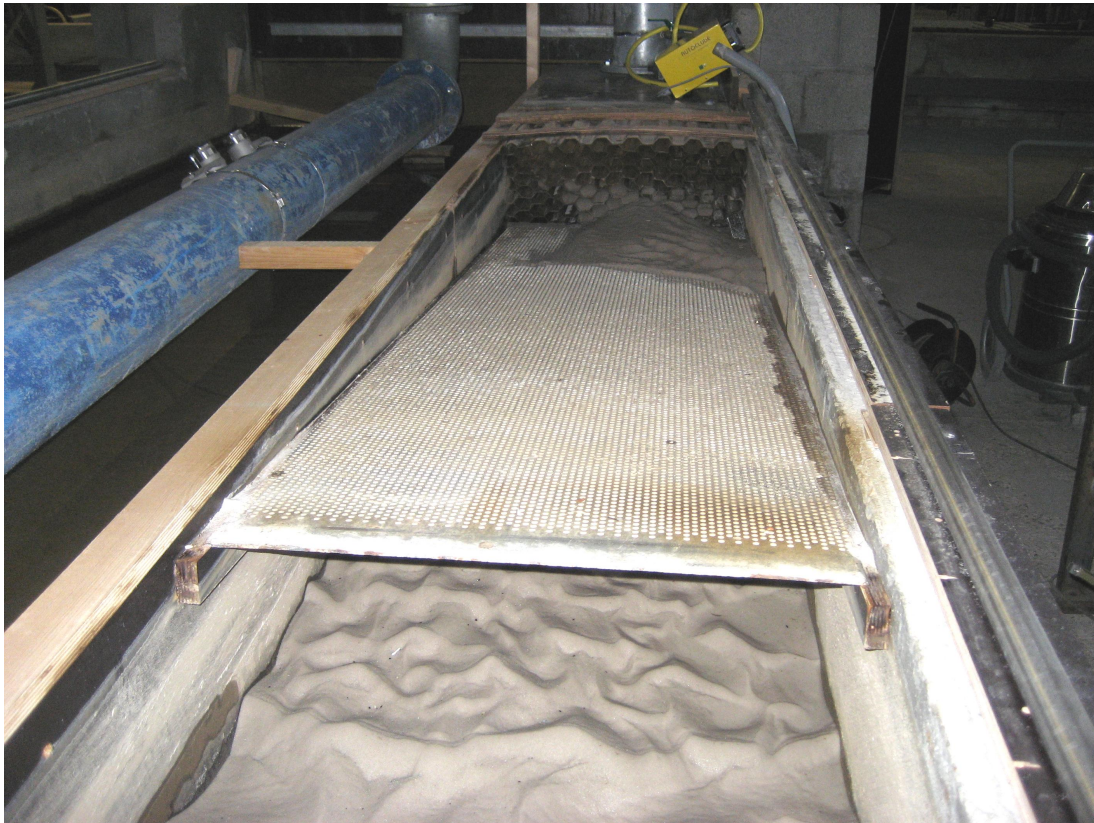
Figure 9 Perforated plate at upstream boundary, looking from downstream
