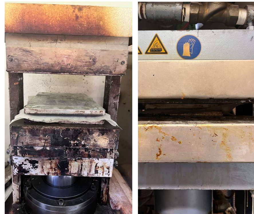
165 °C Heated Contact + 20 °C Cold Press 165 °C for 8 mins + 2.5 Tons 20 °C for 5 mins
