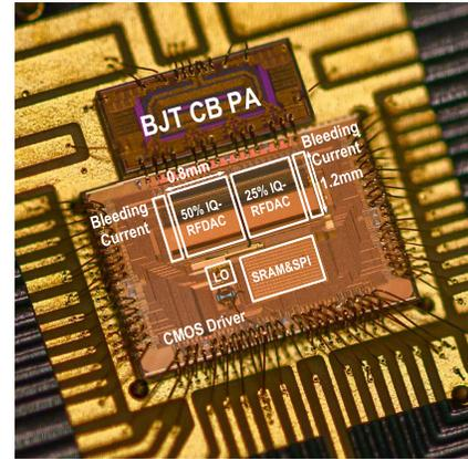
Fig. 15. Chip micrograph of the proposed TX line-up.
