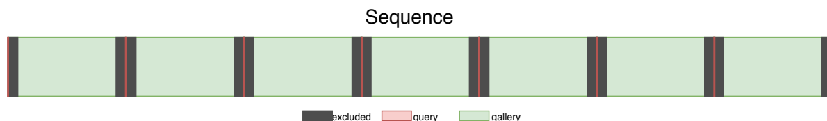
Figure 5.2: Sampling strategy for MatchNMingle-reID query and gallery set. The full rectangle denotes the entire 30-minute video sequence of a particular person. Red indicate the query image, and green indicates the times where gallery images are sampled, and black indicates frames which are excluded.
