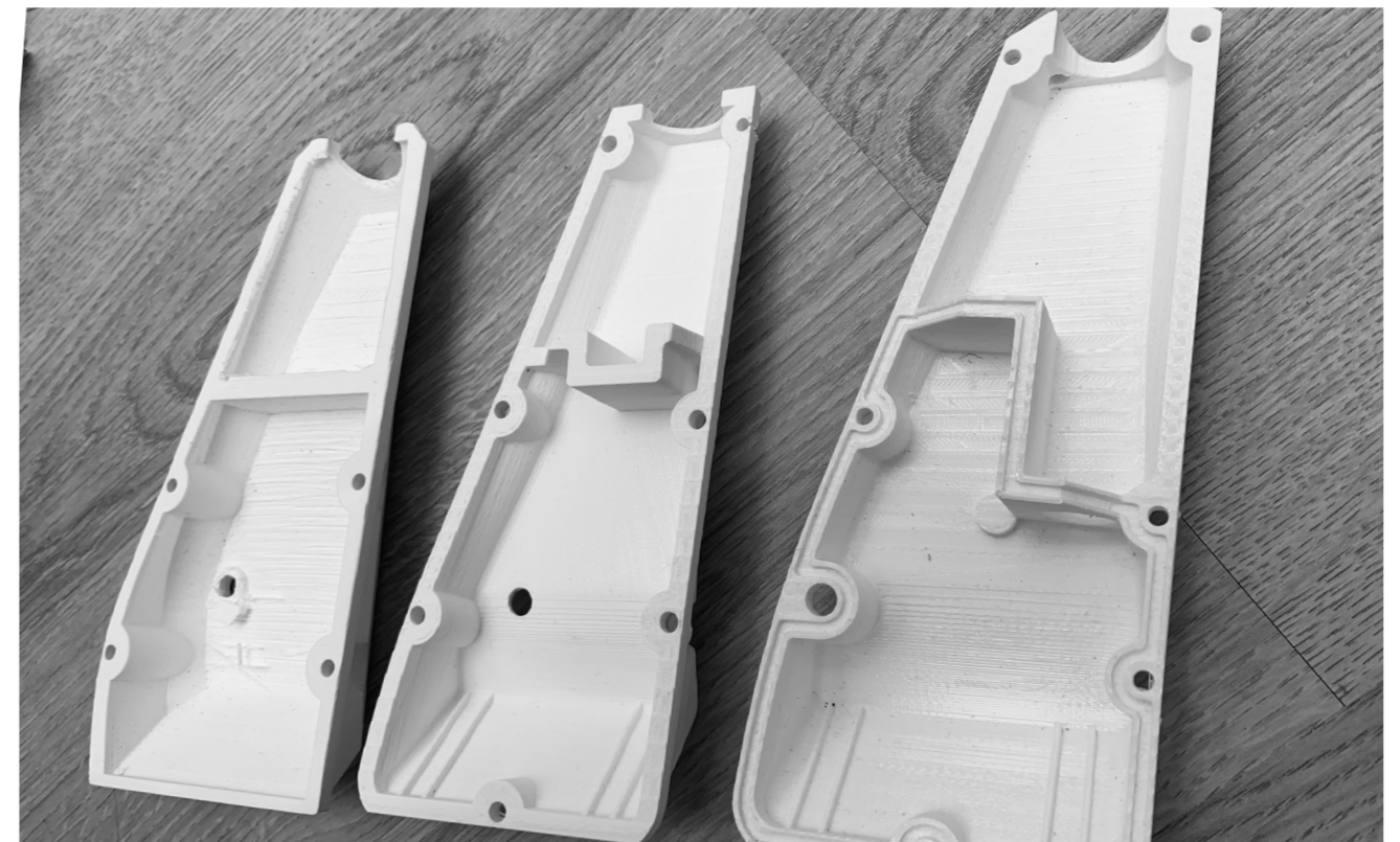
Figure 50: Plastic housing development
