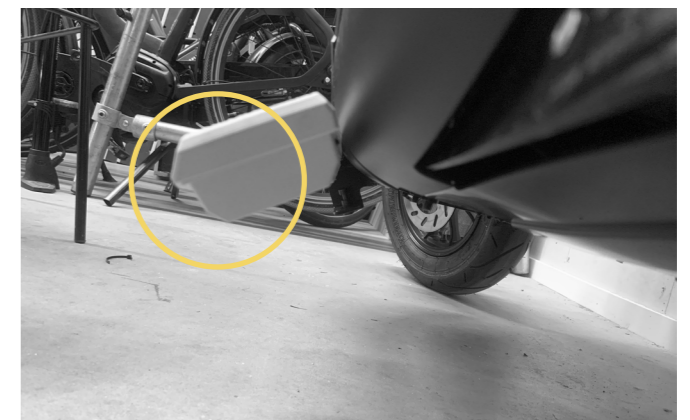
Figure 31: Pictures kickstand sticking out
