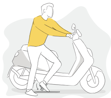
the user will kick out the centerstand above the tile
