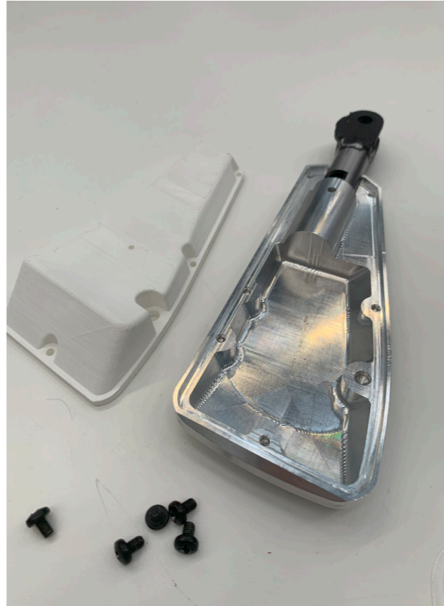
Figure 61: The final aluminum machined housing together with the plastic housing, shaft and screws.
