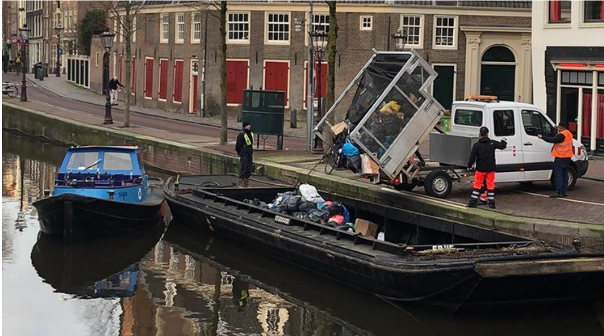
Figure 20. The municipality of Amsterdam is conducting a trial of small garbage trucks that deposit bags into electric boats. This initiative is part of the municipality's search for alternative waste collection methods that can address the current challenges of waste collection in the city centre. Image taken from Gemeente Amsterdam. (n.d.-j).
