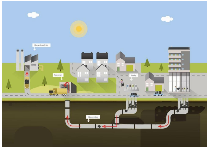
Figure 22. An innovative underground waste transport system is set to be implemented in a neighbourhood in Amsterdam, with the aim of optimising the city's waste management. Image taken from de Brug (2020).
