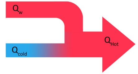
Figure 70 diagram showing that Q_{hot} and therefore COP of heating is always higher than Q_{cold} and cooling COP
