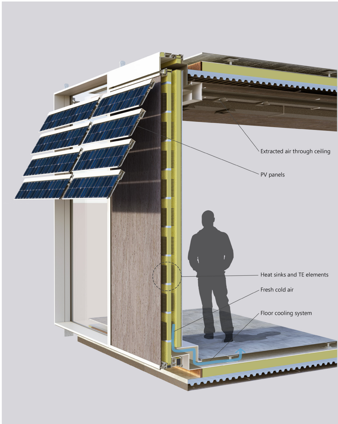
Figure 95 Render showing a vertical section through the TE facade module
