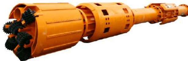
Figure 3.2: Example of a bottom hole assembly for the RCD method [5].
