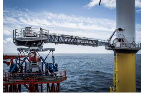
(b) The Ampelmann crew transfer system using a Stewart platform [3].
