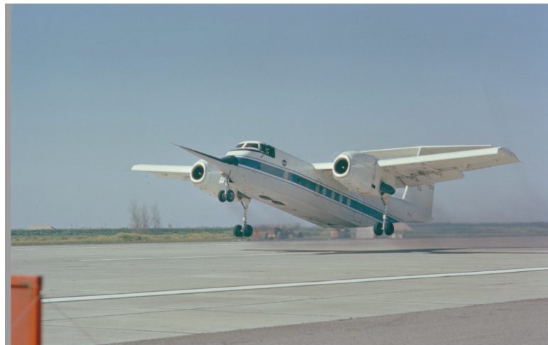
Figure 2.12: NASA Buffalo Augmentor Wing Jet STOL Research Aircraft by NASA, licensed under Public Domain Mark 1.0 .
