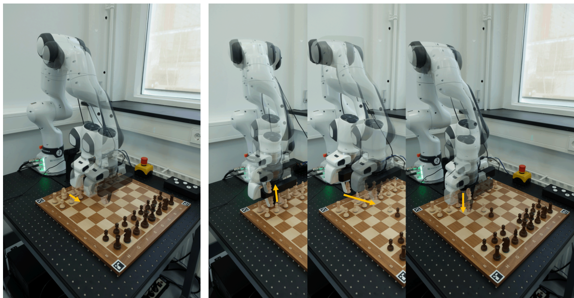
Figure 4.6. The robot is executing planned trajectories to move chess pieces. (A) The robot slides a pawn from the E2 square to the E4 square. (B) The robot lifts the knight on G1 to jump over other pieces on its way.
