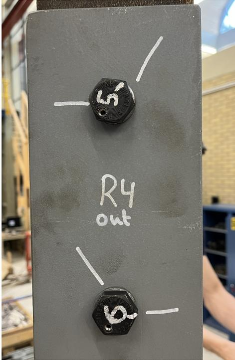
**Figure 6:** Procedure of tightening the bolt by a certain angle, where in this case the bolt head is rotated by 120 degrees instead of the nut. The angle depends on the thickness of the clamping package
