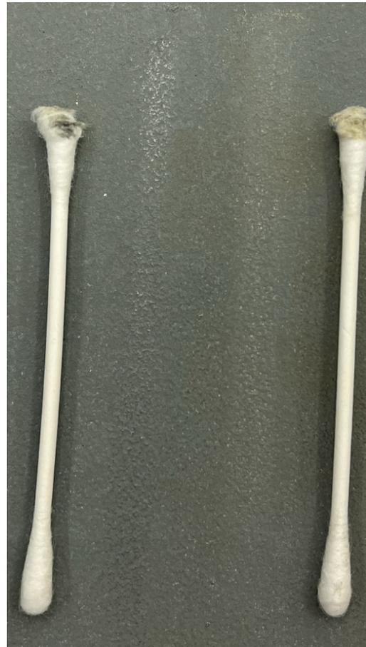
(b) Two types of degradation of the final applied primer after 50 rubs. Left and right path relates to the dry and moist cotton buds respectively
