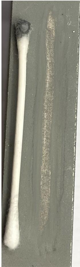
(a) Degradation of the initially applied primer after 21 rubs
