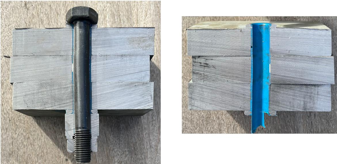
**Figure 52:** Cross-sectional view of a tested IBC
