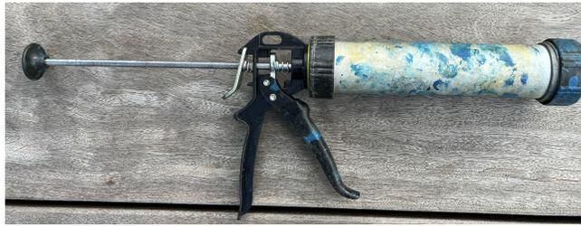
**Figure 9:** Required tool for injecting the resin into the clearing of the connection
