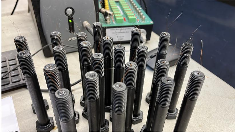
**Figure 35:** M16 bolts after installation of the strain gauges
