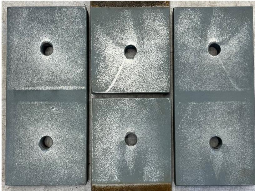
**Figure 46:** Damage on the shear planes of the preloaded bolted connection after the experiment (Specimen R)
