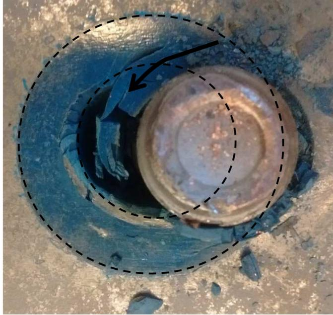
**Figure 74:** Assumed internal shear failure of resin (Nijgh [50])
