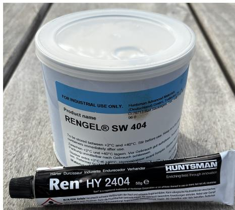
**Figure 10:** Applied two-component-resin with at the back the RenGelSW404 and in front the hardener RenHY2404
