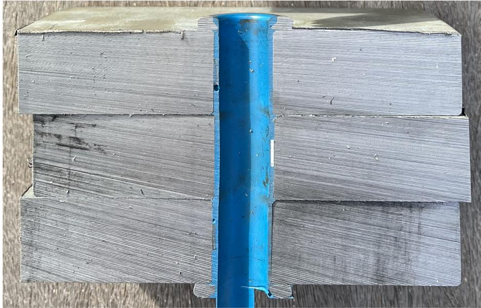
**Figure 99:** Cross-sectional cut of one of the injected bolted connections
