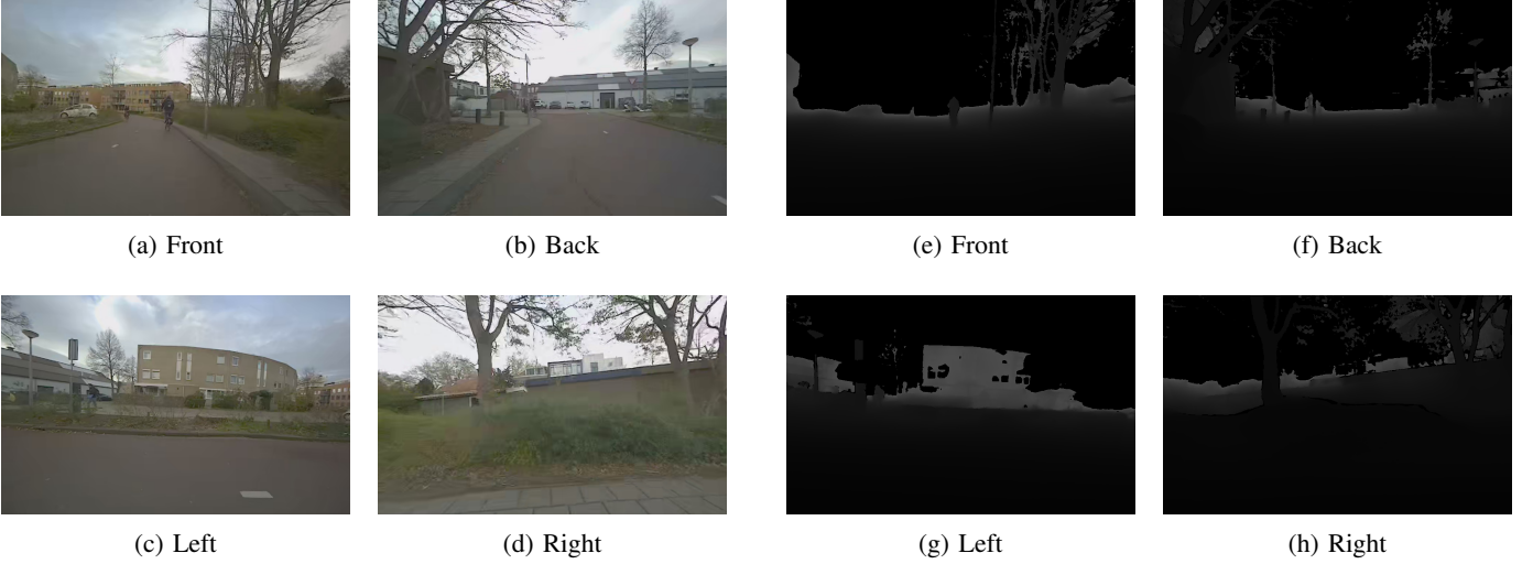
Fig. 4: RGB images taken at the same time instance (a,b,c,d) and their corresponding depth images (e,f,g,h).
