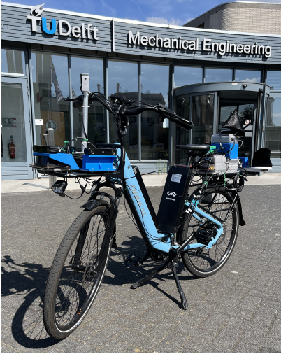
Fig. 3: SenseBike - a data acquisition platform of TU Delft.
