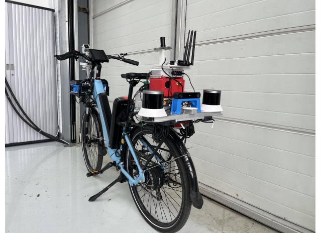
(b) Back camera mount on supporting beam.
