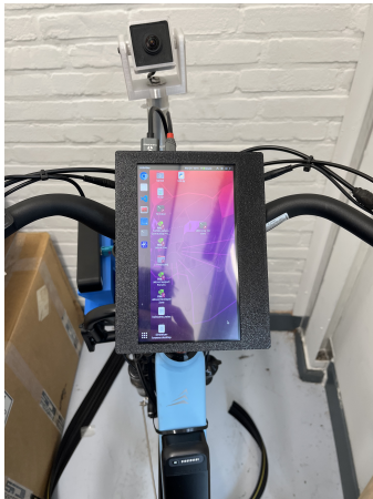
Fig. 8: Control display mounted on a handlebar.
