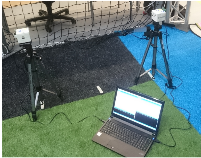
Figure 7-1: Calibrating antenna delays for two UWB modules at 1 meter distance
