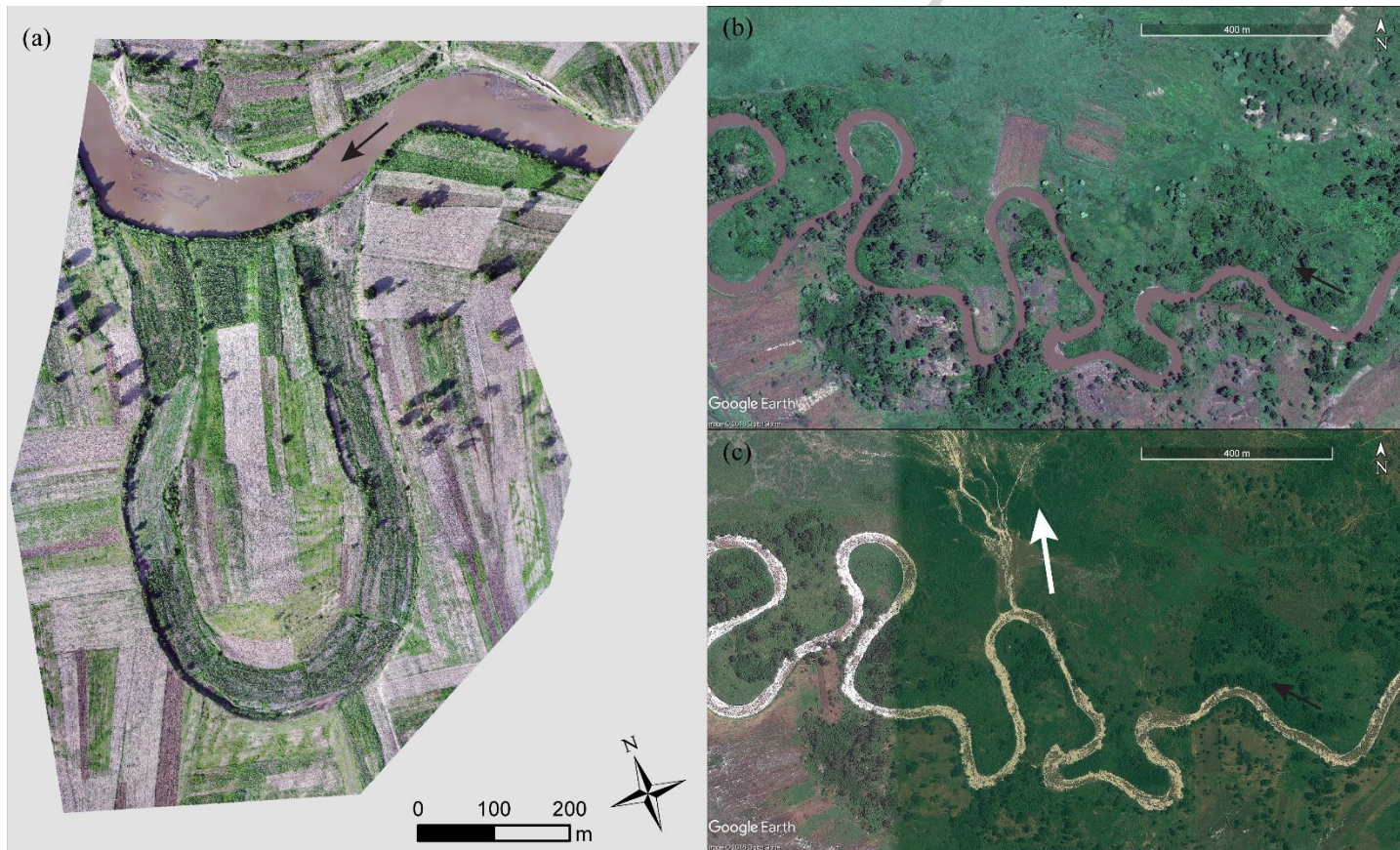
Figure 4 Human activities on river banks lead to bank breaches: a) orthophoto map taken by UAV in November 2017 at CM point showing an old meander cut, heavy farming and no riparian vegetation; b) meandering Mara River near the Pump Station (PM) in 17/01/2010 (Google Earth image); c) same area of b) in 24/09/2010 showing a crevasse in correspondence of a pre-existent crop.
