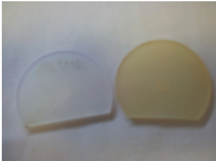
Figure 10: Discoloration of BPA-PC after photo-thermal-ageing at 140 °C
