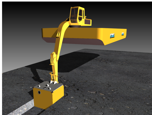
Figure 4.16: CDS with an excavator placed on a pontoon
