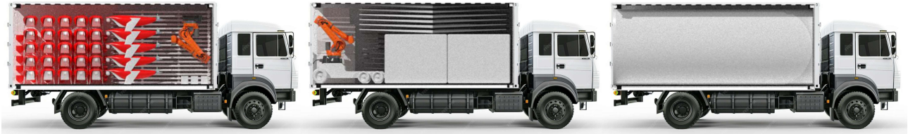
Figure 14.8: Packed ground station
