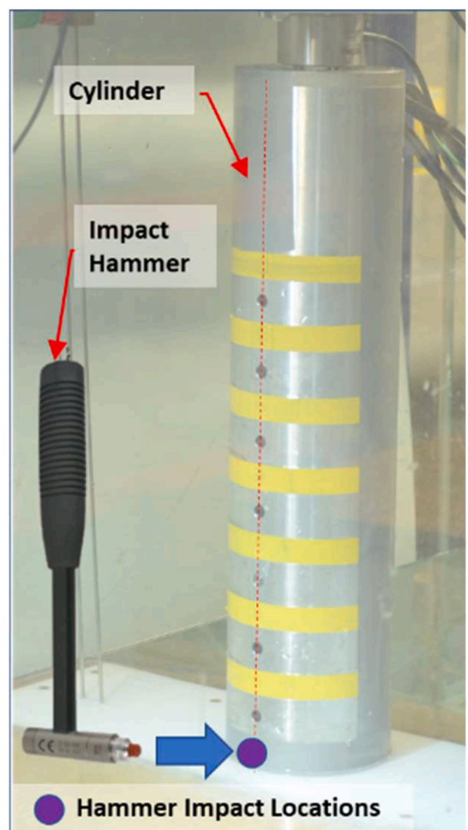
Fig. 14. Impact hammer tests and impact location.
