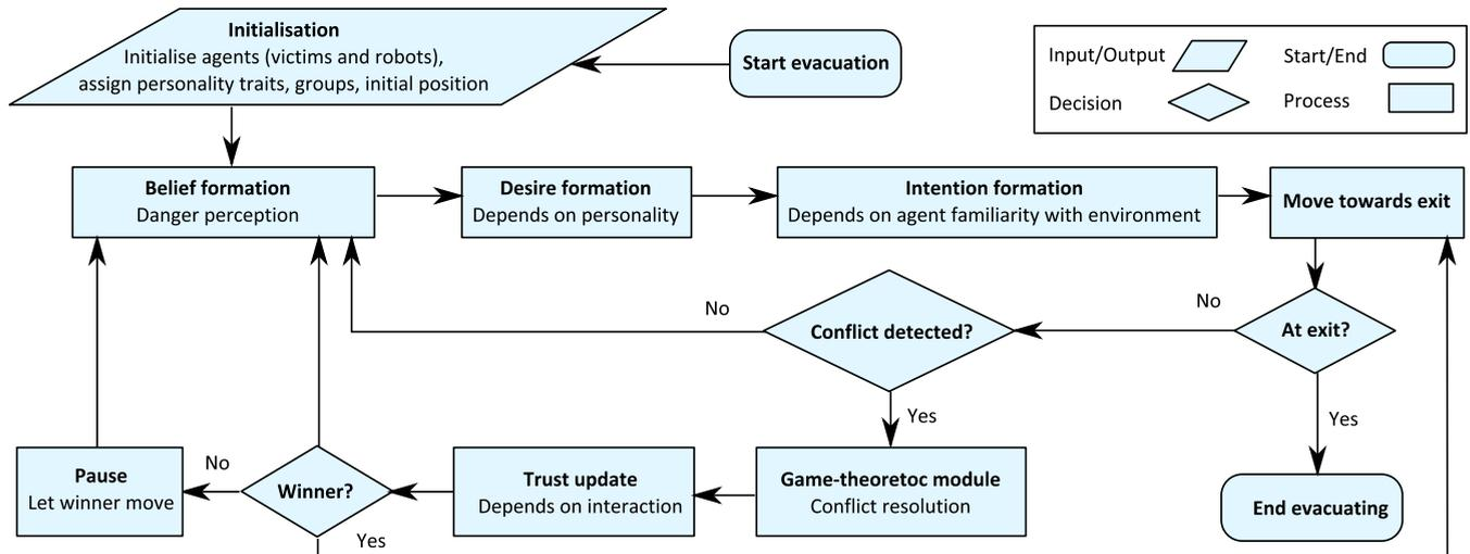
FIGURE 1. Flowchart representing the logic behind the GT-BDI model.
