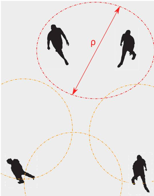
**FIGURE 2.** A conflict occurs and a game is launched whenever at least two agents are in a close neighbourhood of each other (e.g., in a distance equal to or smaller than a given threshold  $\rho$ ). The two agents on top of the figure face a conflict, whereas other agents are outside of the conflict zones of each other.
