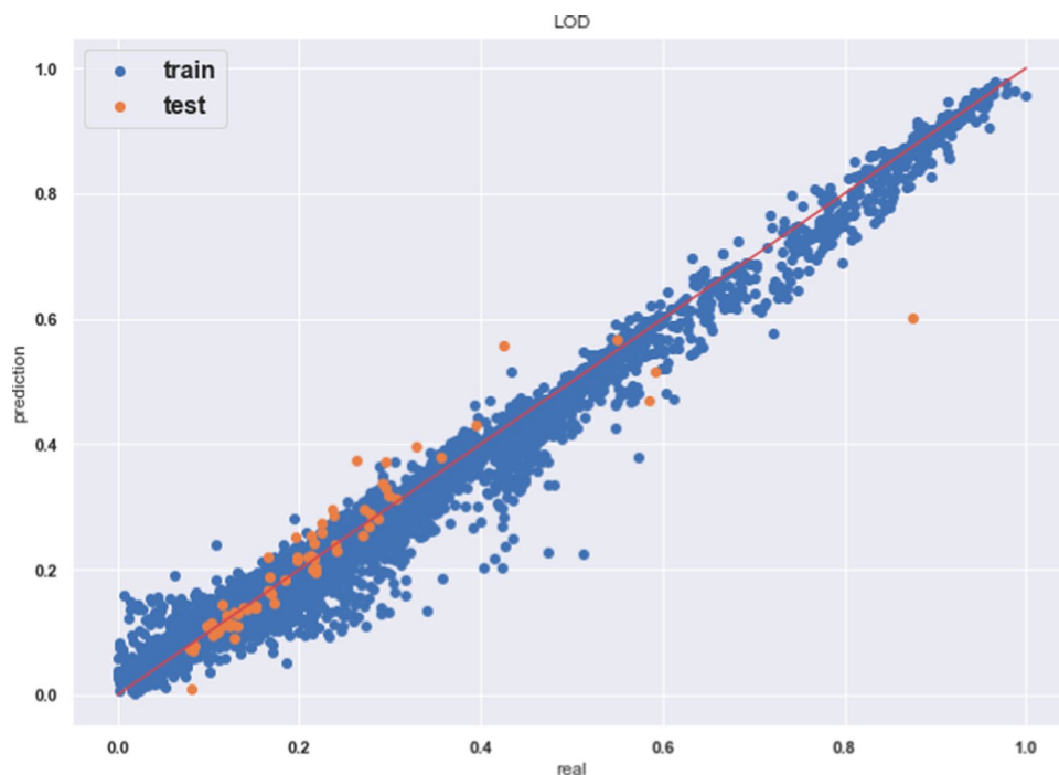
Fig. 6 Normalised ANN (prediction) results versus real values for the Se detection limit LOD. The blue dots are the results for the training set, i.e., the 10,000 synthetic data plus the 80% used for their construction. The orange dots are the results for the 43 real spectra that were not used to generate the synthetic spectra
