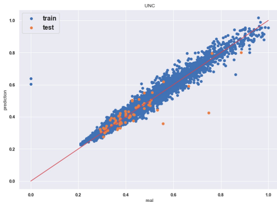
Fig. 5 Normalised ANN (prediction) results versus real values for the uncertainty on the Se content. The blue dots are the results for the training set, i.e., the 10,000 synthetic data plus the 80% used for their construction. The orange dots are the results for the 43 real spectra that were not used to generate the synthetic spectra
