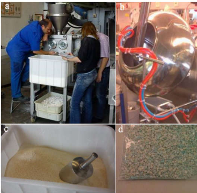
Figure 2.5 a. Roller compaction of powders, b. Coating of particles, c. Uncoated powders and d. Coated powders [1].
