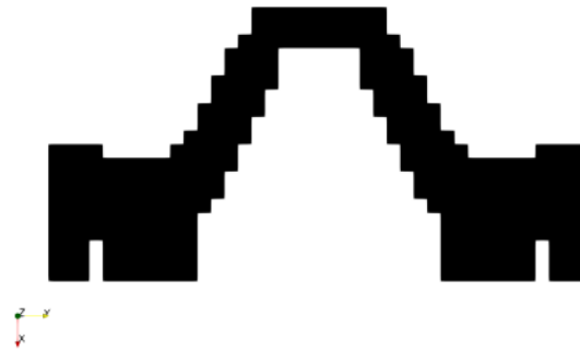
(b) Optimal material distribution with v_f < 0.3
