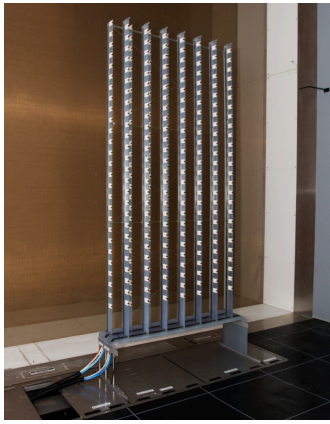
Figure 3.5: Close up of the OJF Seeder inside the settling chamber. Image retrieved from [13].
