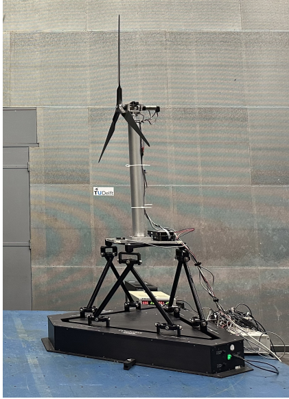
Figure 3.3: DTU 10MW Scale Model and Quanser Hexapod.
