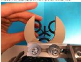
Figure 2: The injected moulded part under the breaking tool.
