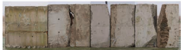
Figure 8 Test wall (side view), dimensions: height=2 m, length=8 m, width=1 m.
