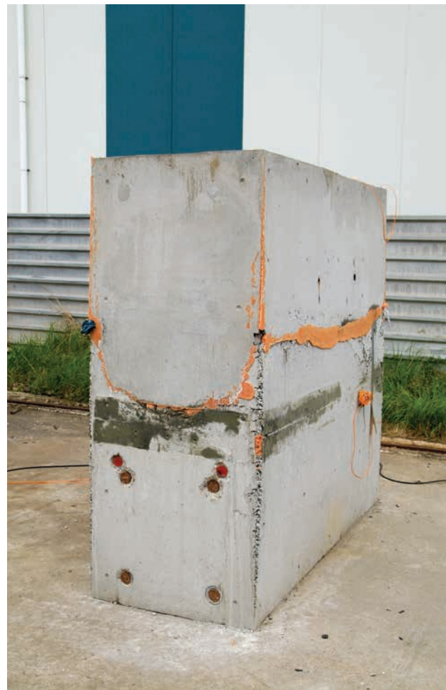
Figure 5 Test block subjected to ER measurement (dimensions: 1*2*2 m 3 )
