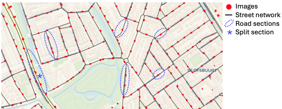
Figure 4.3 Image IDs locations (in red), street network topology (in black) and some road section units (in blue) within a cropped area in Delft, the Netherlands.
