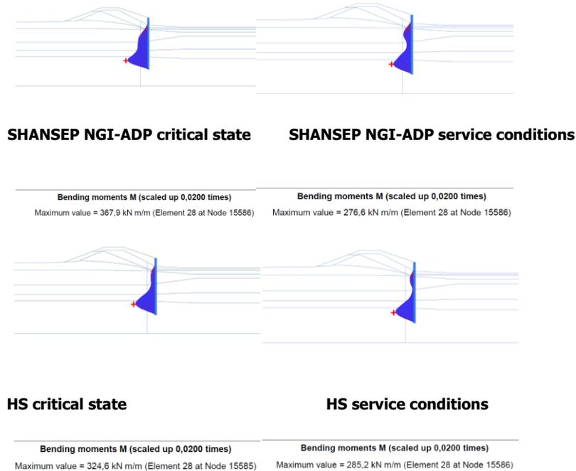
Figure 129: Comparison of moments distribution acting on the sheet pile wall.
