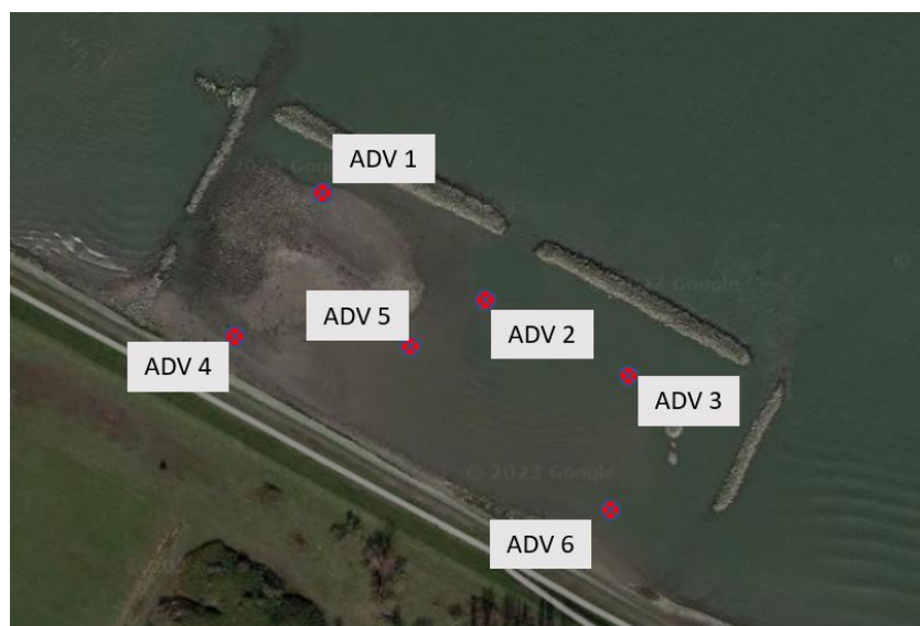
Figure 2.1: Measurement locations of six Acoustic Doppler velocimeters (ADV) (Kouwenhoven, 2023).
