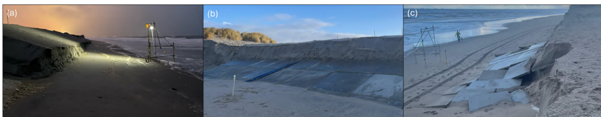
Figure 5.6: Morphological evolution of the hybrid dune (Dike-in-Dune) throughout the experiment, showing changes in dune profile and exposure of the hard core over successive storm events. (a) 19-12-2025, 08:07; (b) 23-12-2024, 11:37; (c) 02-01-2025 15:00
