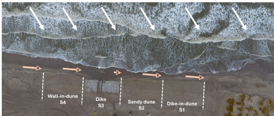
Figure 5.2: Schematic illustration of sediment fluxes under oblique wave conditions. White arrows indicate wave direction; brown arrows show the relative magnitude and direction of longshore sediment transport. The reduced sediment flux in section S3 (Dike-in-Dune) results in a deficit in S2 (Sandy Dune), promoting localized erosion.
