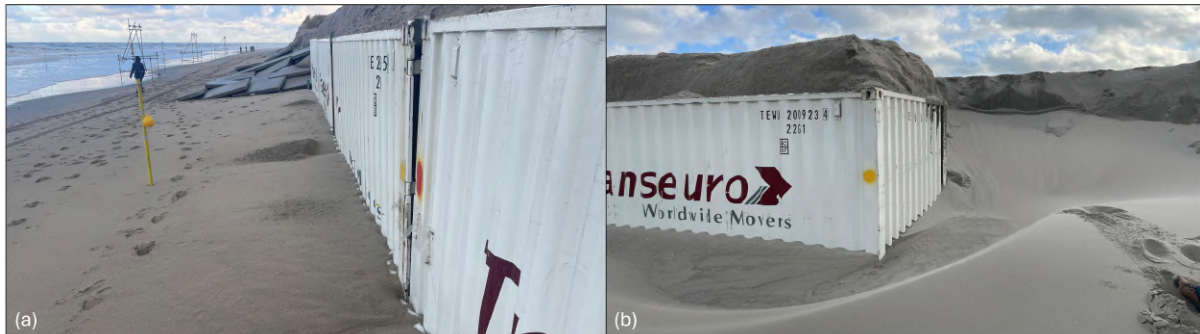
Figure 5.9: Final erosion state of Wall-in-dune (S4). (a) 02-01-2025, 15:08 — Limited toe scour is visible at the base of the container, suggesting wave reflection but no significant undermining. (b) 06-02-2025, 11:29 — The adjacent natural scarp, shaped by wave and wind erosion, retreated further landward following Storms 4 and 5. Backside erosion of the seawall began to emerge.
