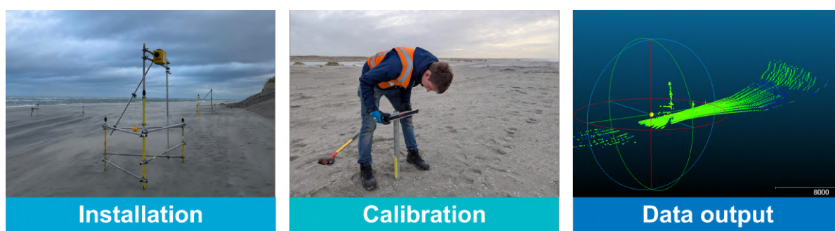
Figure 3.13: Calibration and deployment of the LiDAR system. The left panel shows the frame-mounted LiDAR scanner used during each storm event. The middle panel illustrates the placement of ground control points (GCPs), which were used to align the LiDAR point cloud. The right panel displays the resulting point cloud from a single scan, with all points geo-referenced in the Dutch RD coordinate system.
