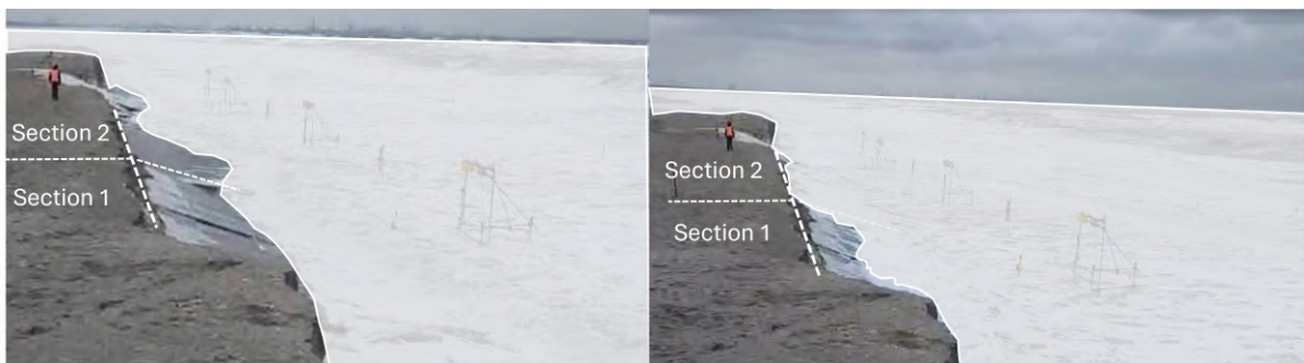
Figure 4.12: Video frames from high water 2.a (22 December, 09:38) illustrating difference in wave runup between Section 1 and Section 2. Left: Wave backwash following a runup event. Right: The wave runup reaches the dune foot in Section 2 (Sandy Dune), whereas it does not reach the dune foot in Section 1 (Hybrid Dune with concrete core), demonstrating the runup-dampening effect of the hard structure.
