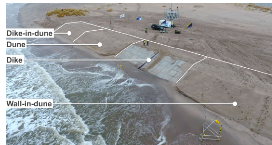
Figure 3.2: The test setup overlaid on an aerial photograph
