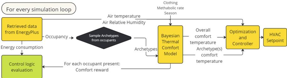
**Fig. 1.** Flow diagram for occupant-centric control logic.
