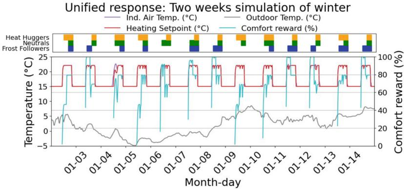
**Fig. 3.** Two-week simulation for occupant-centric control logic: Unified response. The plot presents how the heating setpoint changes air temperature, and the comfort reward shows the (miss)alignment between the occupant archetype (top figure, blanks mean unoccupied) thermal preference and the air temperature. The climb of the comfort reward at the beginning of the occupied time is due to the delay in heating the space from 15 °C.
