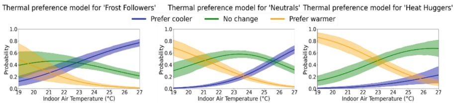
**Fig. 2.** Thermal preference posteriors for **a.** *Frost Followers* **b.** *Neutrals*. **c.** *Heat Huggers*. In relation to indoor air temperature, with other features considered at mean values. Blue, green, and orange areas represent the mean and standard deviation of the probability of being in one of those three classes, preferring cooler, no change, or warmer, respectively.
