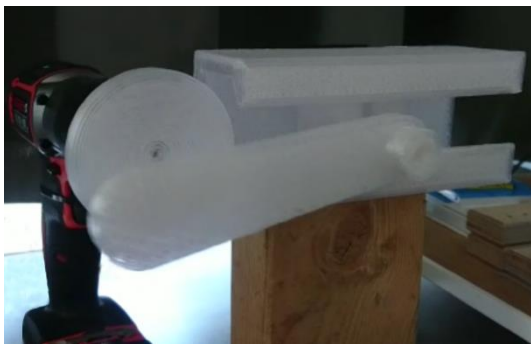
Figure 40: Wear test setup with printed elements and electric drill
