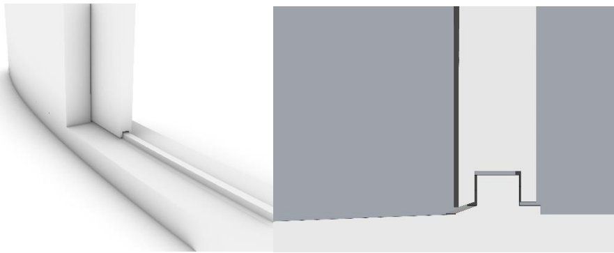
Figure 20 side profiles of raised rail with panel
