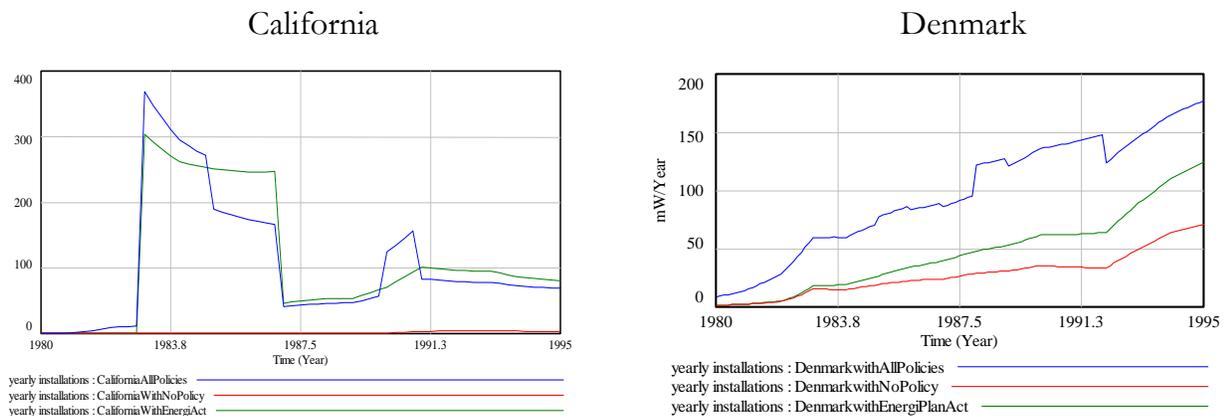
**Figure 7.6 Effect of EnergiPlan Act on wind turbine installations**
