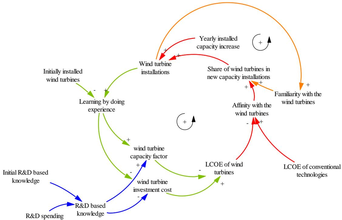
**Figure 5.5 Conceptual Diagram of Wind Turbine Diffusion Model**
