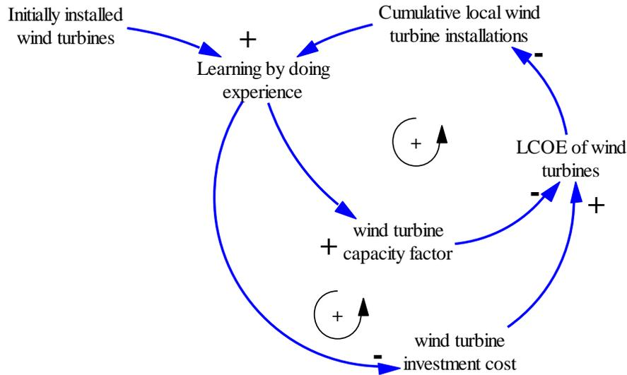
**Figure 5.2 Learning by doing mechanism in wind turbine diffusion**
