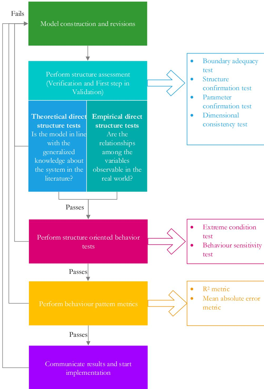
Figure 6.1 Verification and Validation Design (Barlas, 1996; Sterman 2000)
