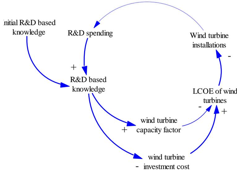
**Figure 5.3 Learning by searching mechanism in wind turbine diffusion**
