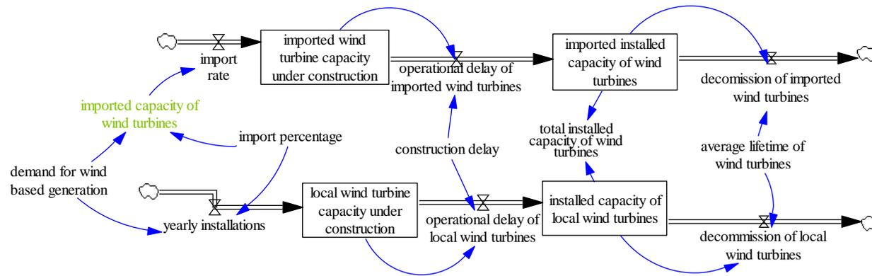
**Figure U.4 Installation of wind turbines**
