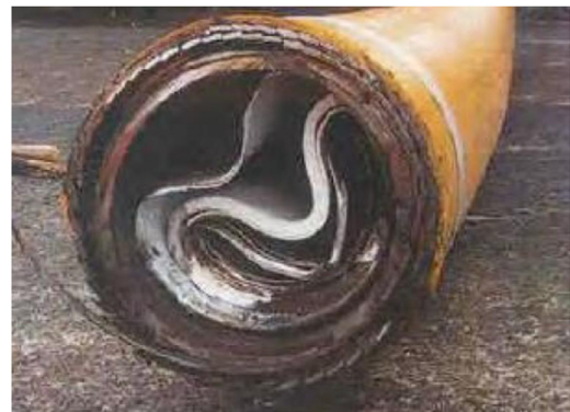
Fig. 3. Collapse failure of the flexible riser [11].
