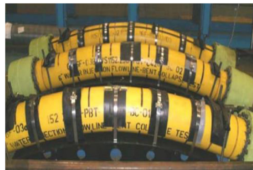
Fig. 7. Curved collapse test samples [21].
