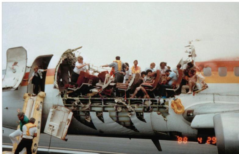
**Figure 2-4:** Aftermath of the accident of flight 243, which was caused by a fatigue failure originating from multiple locations (source: [www.nytimes.com](http://www.nytimes.com))
