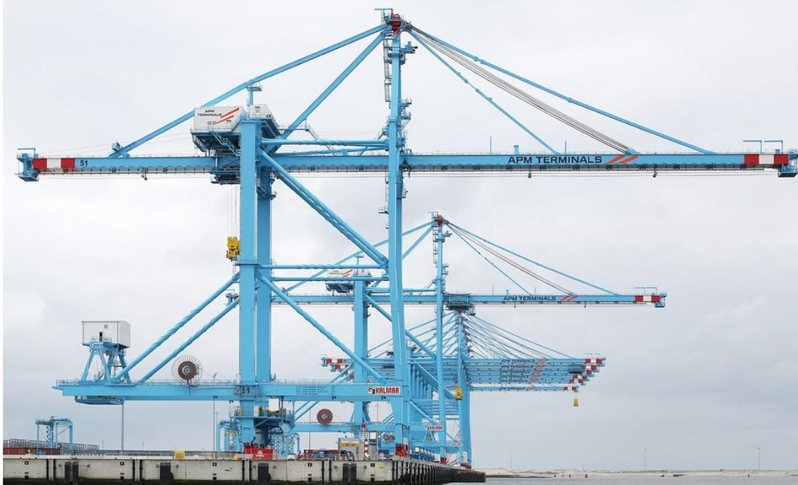
**Figure 1-1:** Example of a STS gantry crane (source: [www.flickr.com](http://www.flickr.com)).
