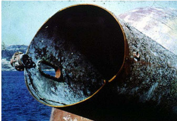
**Figure 8-4:** The brace which failed as a result of a fatigue crack originating from the hydrophone support, which is still attached to the wreckage (source: [www.olechris.page.tl](http://www.olechris.page.tl)).
