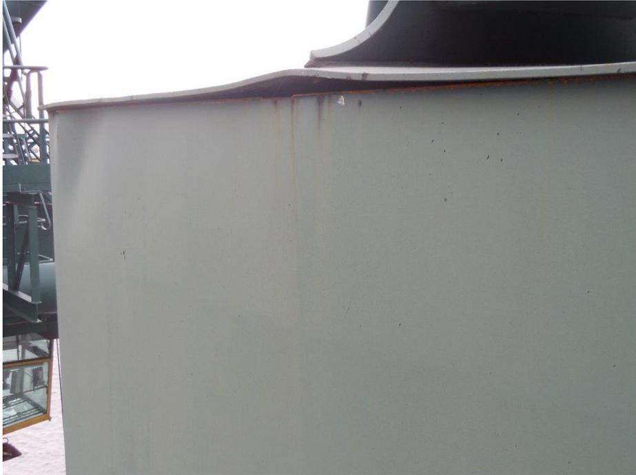
**Figure 4-6:** Example of large deformations as a result of a fatigue crack. LEFM models are not valid in this case (image provided by Cargotec).
