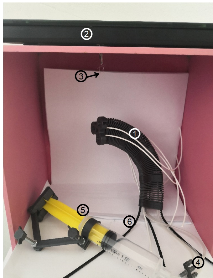
Fig. 16: Picture of the operating force test setup. The prototype (1) is attached to the scale (2) with a cable (3). As the shaft assumes several configurations the air tubes (4) are expanded with a syringe (5). The shaft is then pulled down until a timing belt (6) tooth starts slipping across the stopper.
