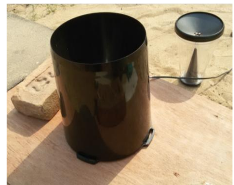
Figure 20: The placement of the tipping bucket and the manual rain gauge at the ITC
